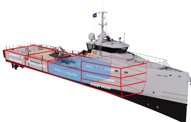
Figure 3. Examples of spaces assigned to their compartments overlaid on the VSX5209.
