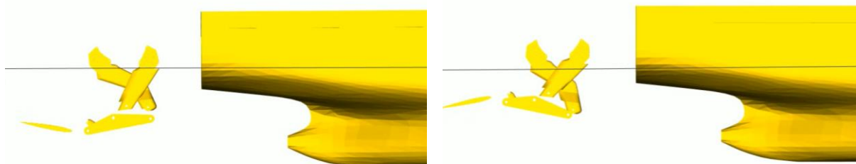
Fig.3: WaveDrive fin system in waves in operation (snapshots of simulation)
