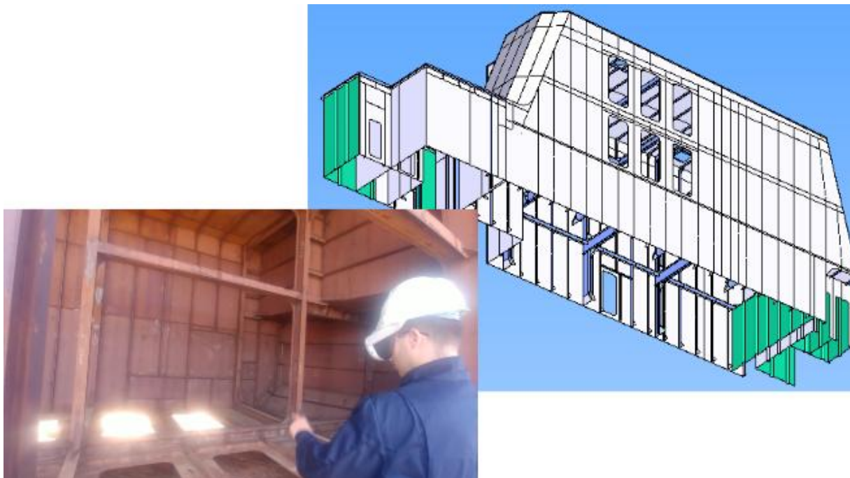
Fig.2: 3D model and preparation for inspection of the finalized hull building block (45t steel funnel)
