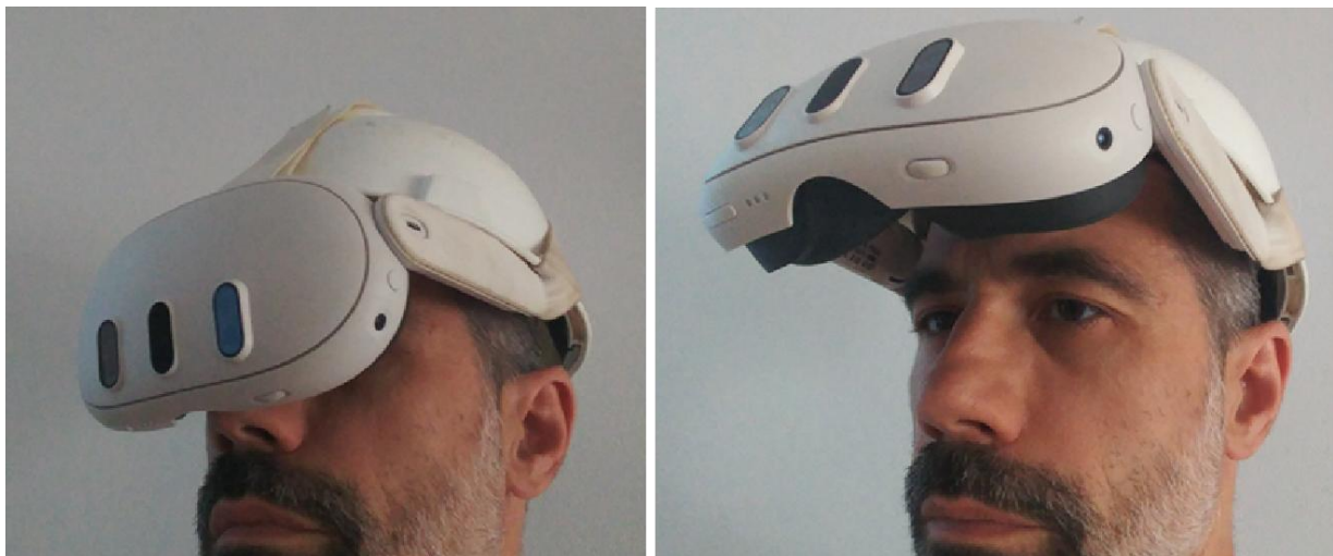
Fig.1: Adjustable position of the HMD on a protective helmet allowing clear sight without removing
