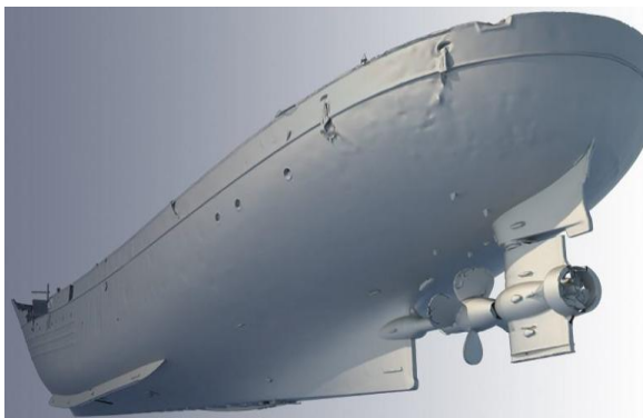
Fig.3: 3D underwater scan of ship hull
