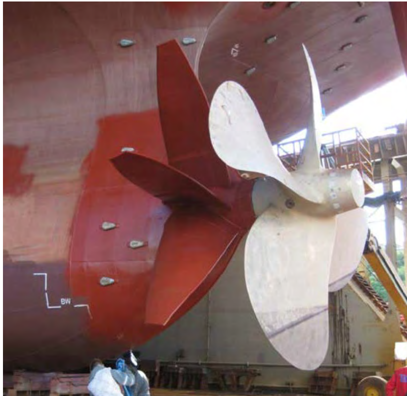
Fig.2: Pre-Swirl Stator (PSS) installed in the dry dock
