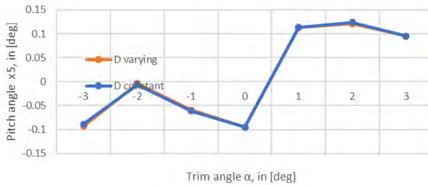
Fig.7: Simerics-MP calculations for pitch free-motion at 14 kn for different trim angles
