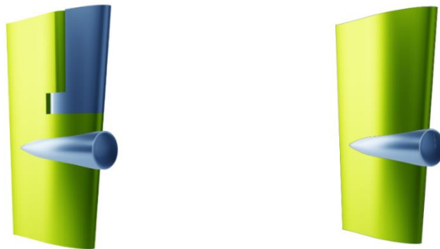
Fig.13: Rudders generated parametrically within CAESES
