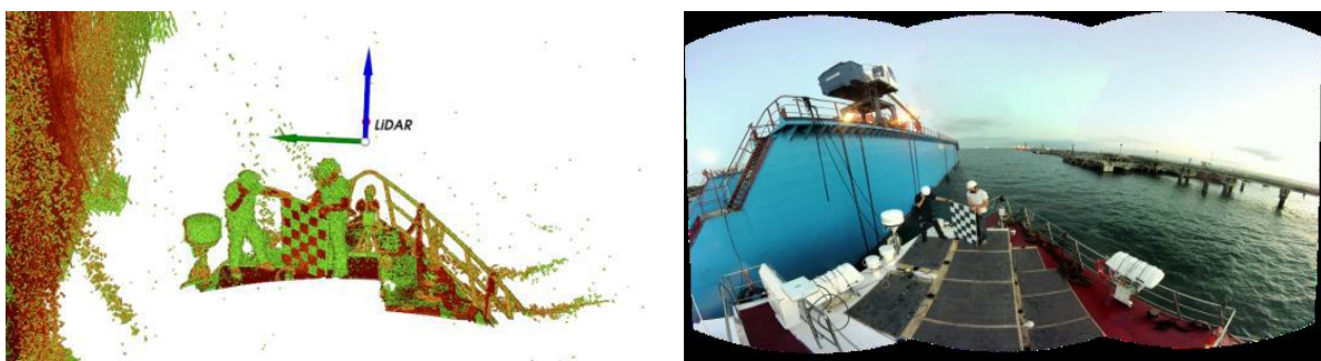
Fig.9: Example of point clouds by LiDAR acquisition and stitched image by elaborating bow pod data
