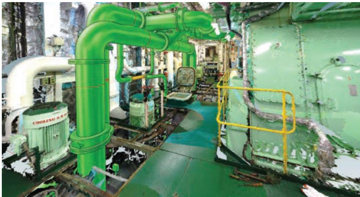
Fig.6: Laser data integrated with 3D model in E3D Design
