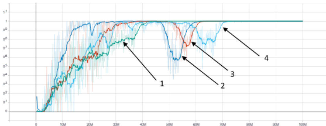
Fig.6: Success ratio of different actuator configurations during training. Duration 100 million steps. Zero means no episode was successfully completed, one means all episodes were successfully completed. 1: Side by side arrangement with 5 target points. 2: Skew arrangement. 3: Line arrangement. 4: Side by Side arrangement Standard Training.
