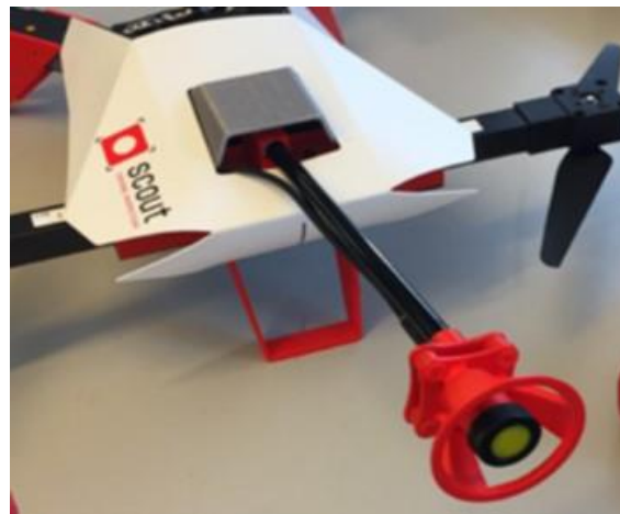
Fig.5: Drone carrying ultrasound sensor for thickness measurements – UTM (courtesy by Scout Drone Inspections)
