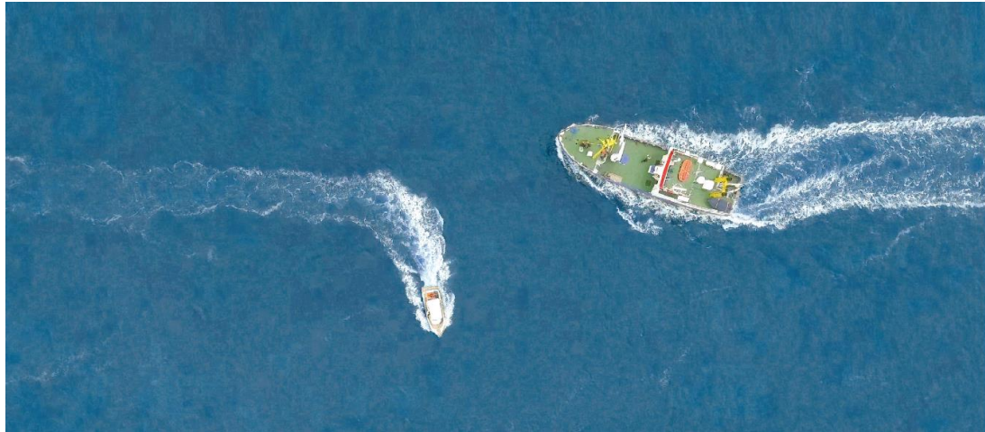
Fig.5: Zuse (left) and Senckenberg (right) performing an evasive manoeuvre recommended by MTCAS during the field test in the Innenjade
