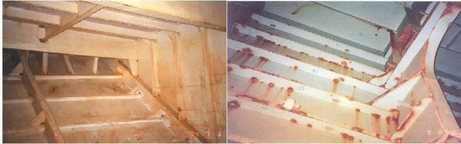
Fig.3: Examples of coating condition and corrosion; GOOD (left); FAIR (right)
