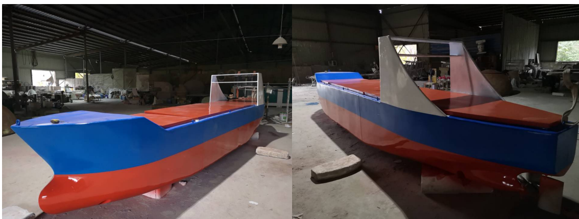
Fig.4: A new 7 m long KVLCC2 model ship for remote-control and autonomous navigation tests
