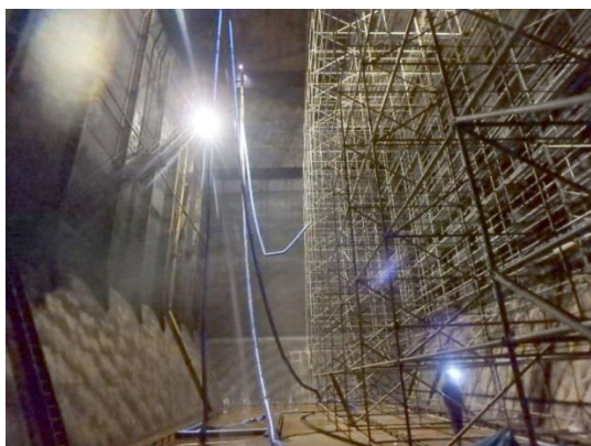
Fig.1: Staging erected for accessing and surveying bulkhead of cargo hold (left); ballast tank with high number of bays to be examined during survey (right)
