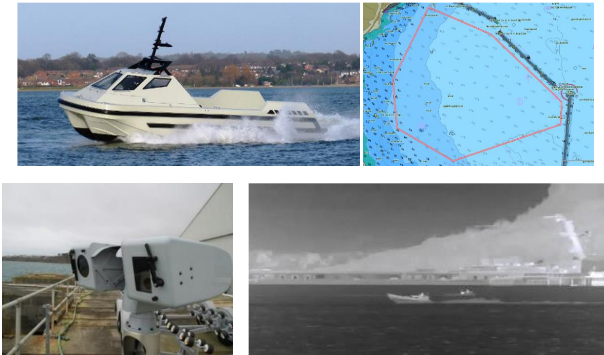
Fig.7: ARCIMS USV (top-left); sea-trial controlled environment (Bingley/UK) (top-right); Electro Optical camera (bottom-left); EO image (bottom-right).
