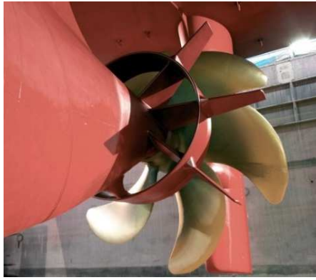
Fig.10: Twisted fin as typical PDI Source: Becker Marine
