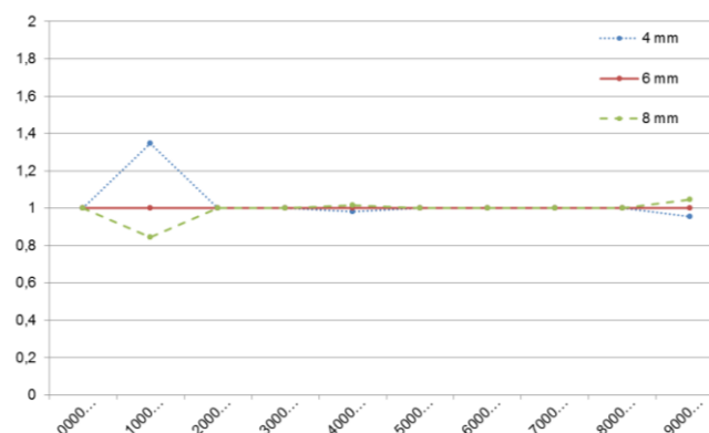
Fig.5: Analysis of effect of plate thickness on production work content per SWBS category, Sigma 10514
