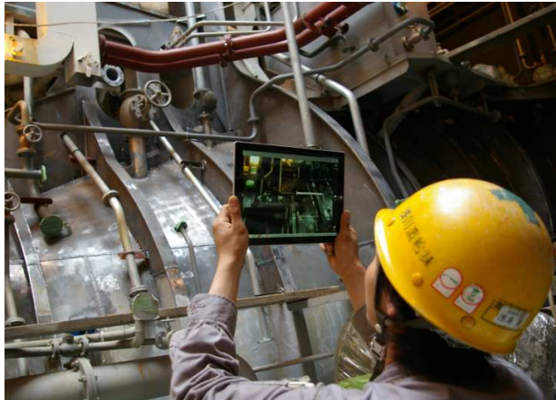
Fig.21: Augmented Reality in ship construction, source: Matsuo Kohei (NMRI)
