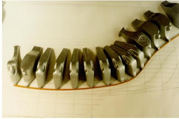
Fig.4: Traditional splines for ship design, source: TU Berlin
