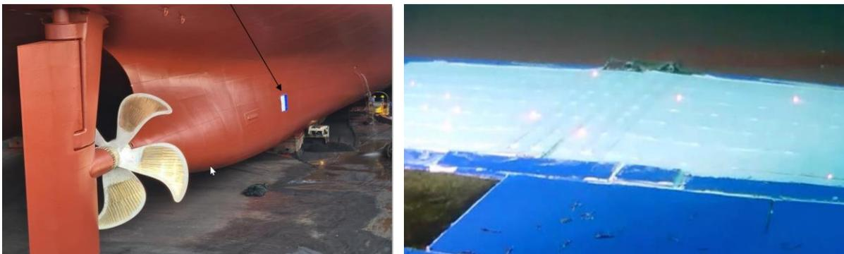
Fig.8: Tile installation on LNG carrier (left), panel performance after 12 months (right)
