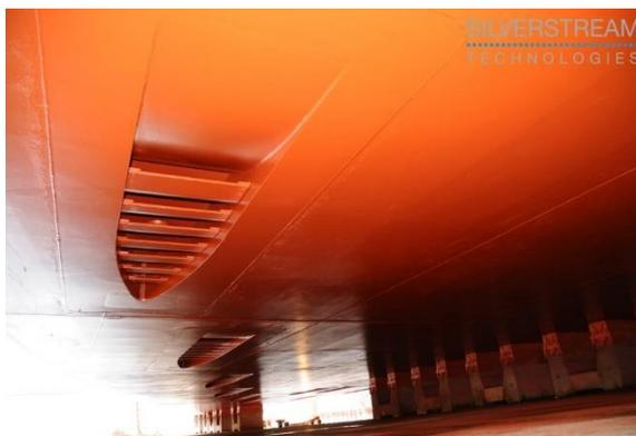
Fig.14: Air lubrication system, source: Silverstream Technologies
