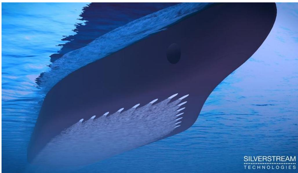
Fig.1: Ship hull bottom coated with air bubbles released from the Air Release Units (ARUs)
