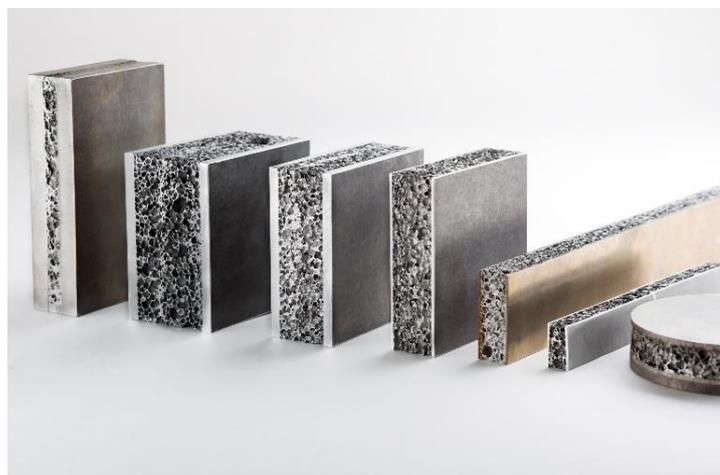
Fig.1: Example of a steel-aluminium foam-steel sandwiches with overall thickness of 35 mm (3/29/3) (left) and different samples (right)
