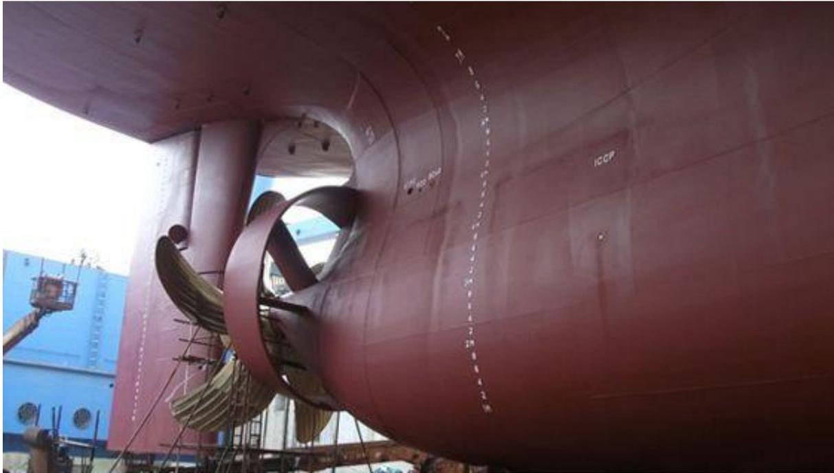
Fig.6: Mewis duct as example for a PID, source: Oldendorff Carriers
