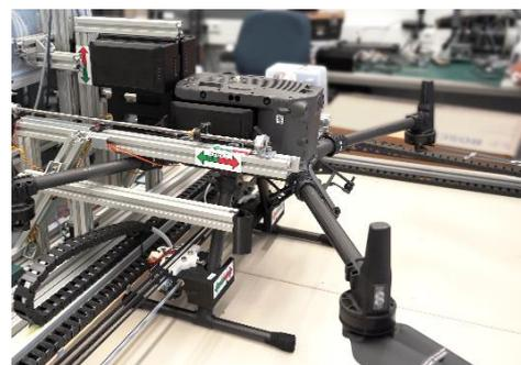
Fig.13: Step 6 - BSS unlocks battery safety lever and swaps left side battery
