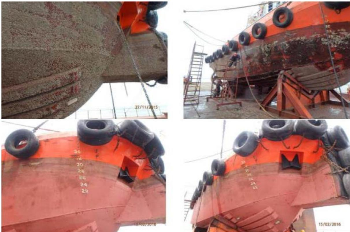
Fig.8: Tugboat without (top) and with (bottom) ultrasonic antifouling protection
