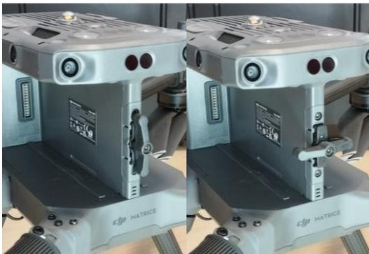
Fig.6: Empty battery slots of M300 with battery safety lever in unlocked (left) and locked (right) position. Clearly visible is the battery contact in the back at the vertical wall and a guiding rail at the bottom of the compartment, on which the battery slides onto.
