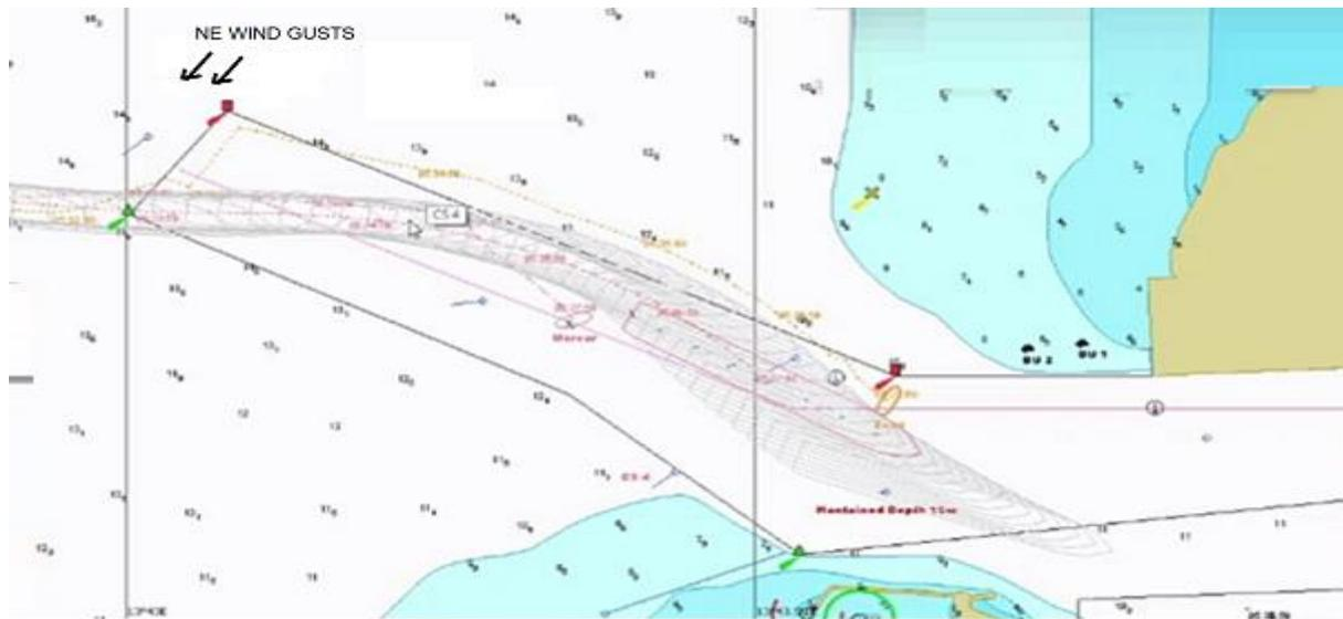
Fig.1: Port of Koper-approach to the container terminal. The ship entered the canal at an undesirable angle due to wind gusts and the participant's late reaction. Two tugs assisted the 14 m draft container ship stay on course within the dredged channel.
