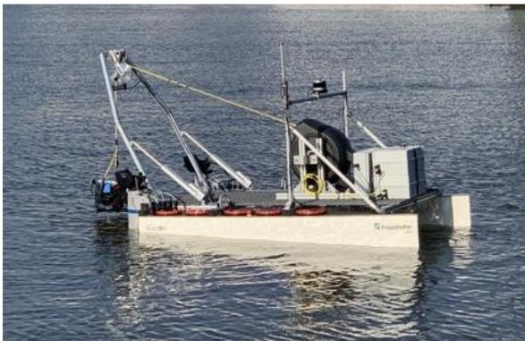
Fig.2: ASV SeaLion in underwater inspection configuration. The ample deck space incorporates an ROV to perform ship and quay wall inspections. The implement domain (grey box) at the front will remain in the UAS configuration.
