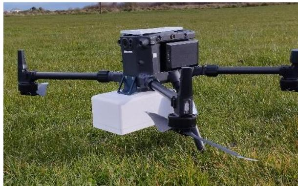
Fig.3: M300 equipped with one of the RAPID payloads – ship emission system MESU (Mobile Emission Sensory Unit), developed by CML to measure up to six gaseous emission products.
