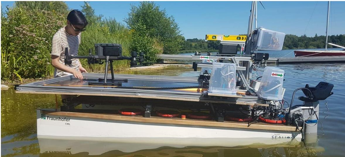
Fig.16: The first setup where the BHS is centered on SeaLion. The landing platform has an inclination of  $1.8^\circ$  before the adjustment.
