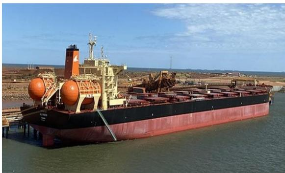
Fig.17: LNG as fuel installation on bulk carrier “HL Green”
