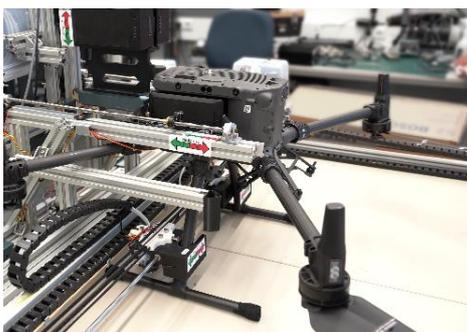
Fig.12: Step 4 - DPS positions drone inside the BSS
