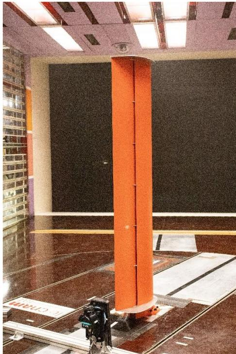
Fig.2: Scale 1:4 model of the asymmetric CWS wingsail in the IAT wind tunnel
