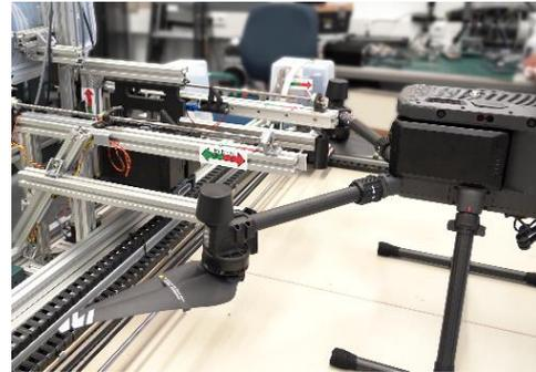
Fig.15: Step 12 - DPS positions drone on platform in takeoff position
