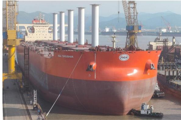
Fig.16: WASP installations on bulk carriers
