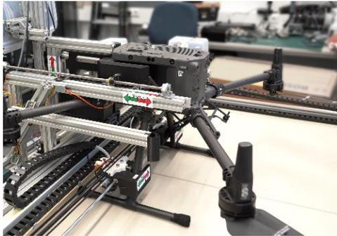
Fig.14: Step 8 - BSS swaps right side battery and closes battery safety lever
