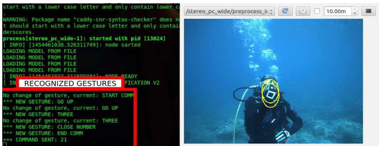
Fig.18: Gesture recognition in CADDY diver support robot, http://www.caddy-fp7.eu/
