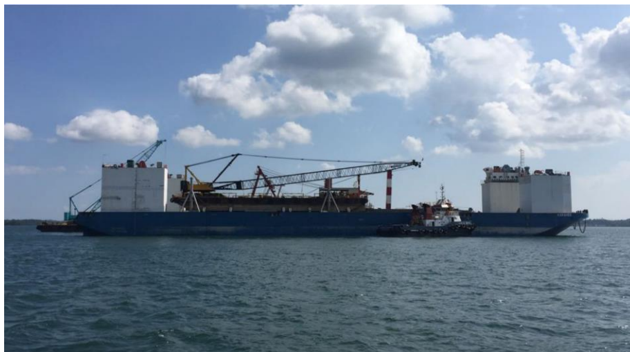
Fig.14: The 122 m LOA heavy lift barge has a 28000 t lifting capacity
