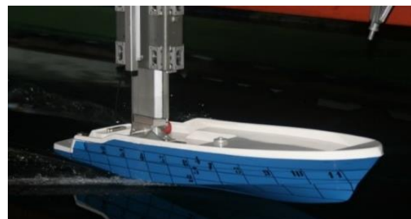
Fig.4: Towing tests at DII tank of parent non monohedral hull form
