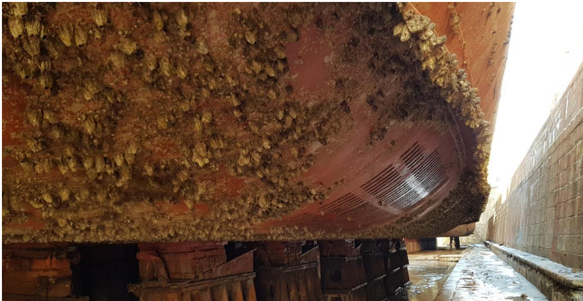
Fig.5: Sea Chest view from outside after 3.5 years in operation with DBP
