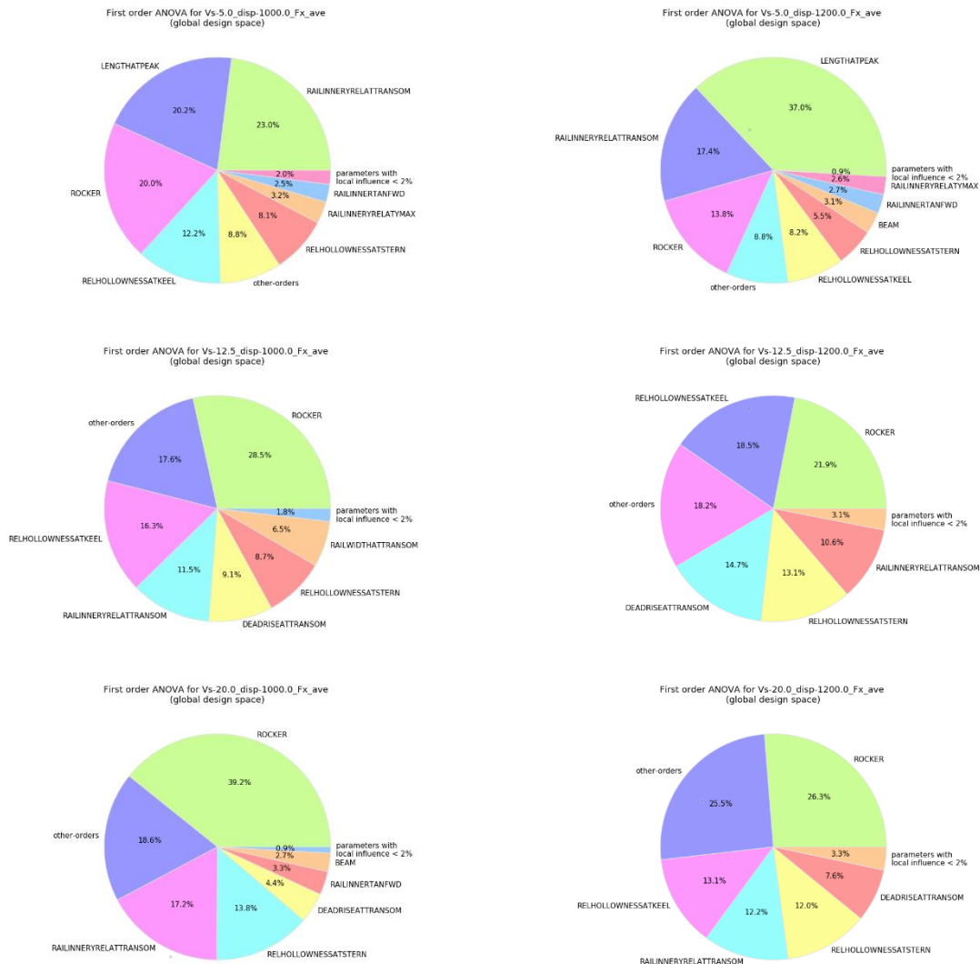
Fig.19: ANOVA: left 1000 kg, right 1200 kg, top to bottom: 5 m/s, 12.5 m/s, 20 m/s
