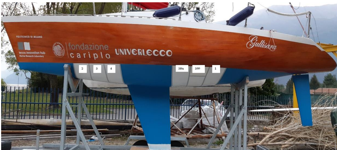
Fig.2: The order of test samples on the Testing hull
