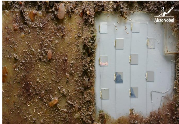
Fig.12: UV-based antifouling, source: AkzoNobel
