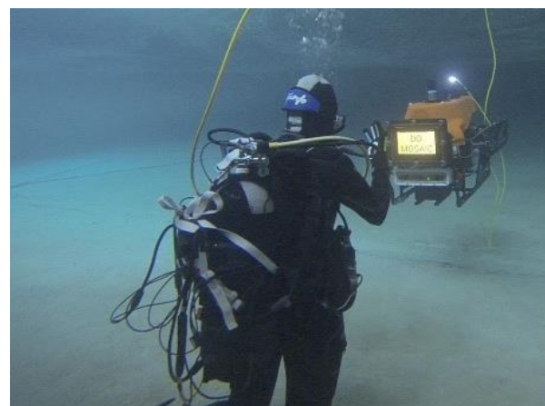
Fig.17: CADDY robot acknowledging diver command to do mosaic
