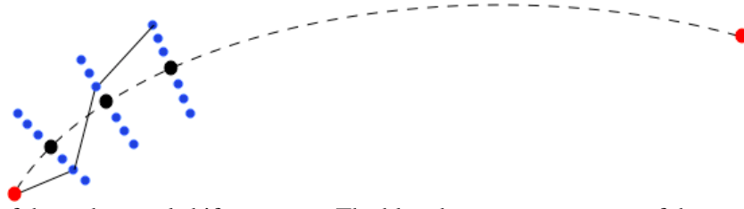
Fig.15: Sketch of the orthogonal shifts concept. The blue dots represent some of the potential orthogonal deviations from the Orthodromic route (represented by a non-continuous curve).
