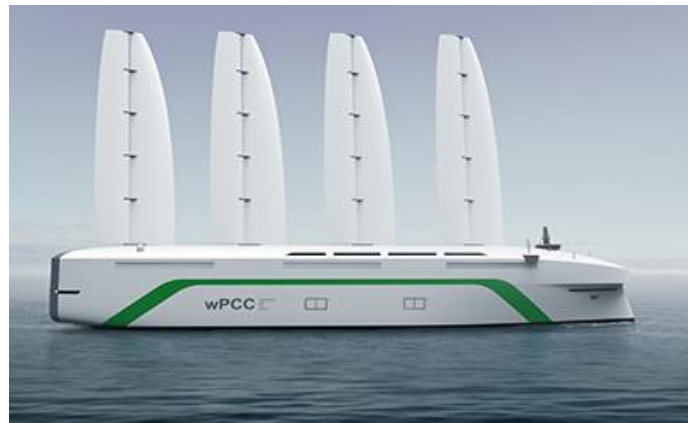
Fig.2: Wind-power car carrier, developed jointly by KTH Stockholm, SSPA Gothenburg and Wallenius Wilhelmsen
