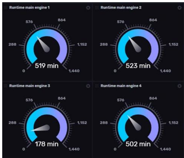
Fig.7: Runtime visualisation of the main engines using the Influx database UI
