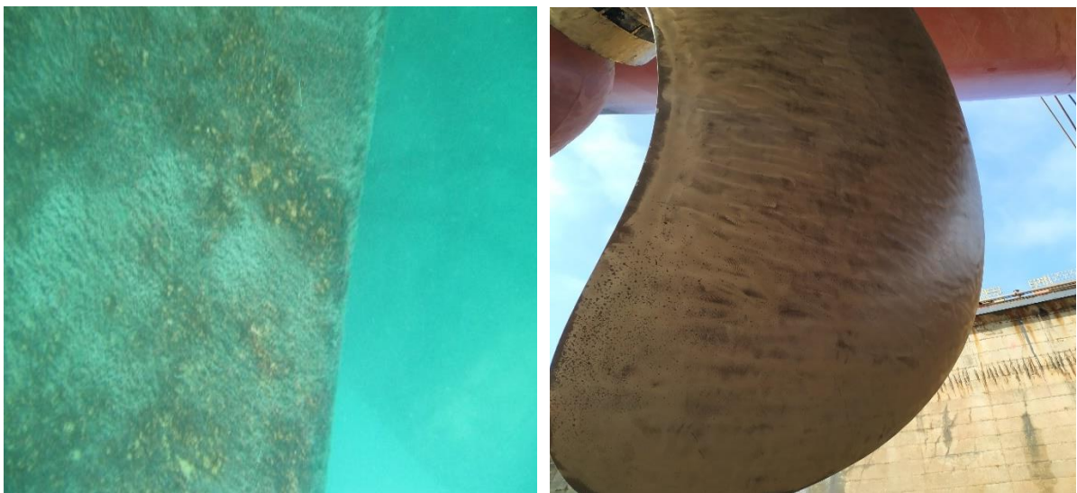
Fig.6: Propeller after 6 months without DBP and comparable propeller after 3 years with DBP
