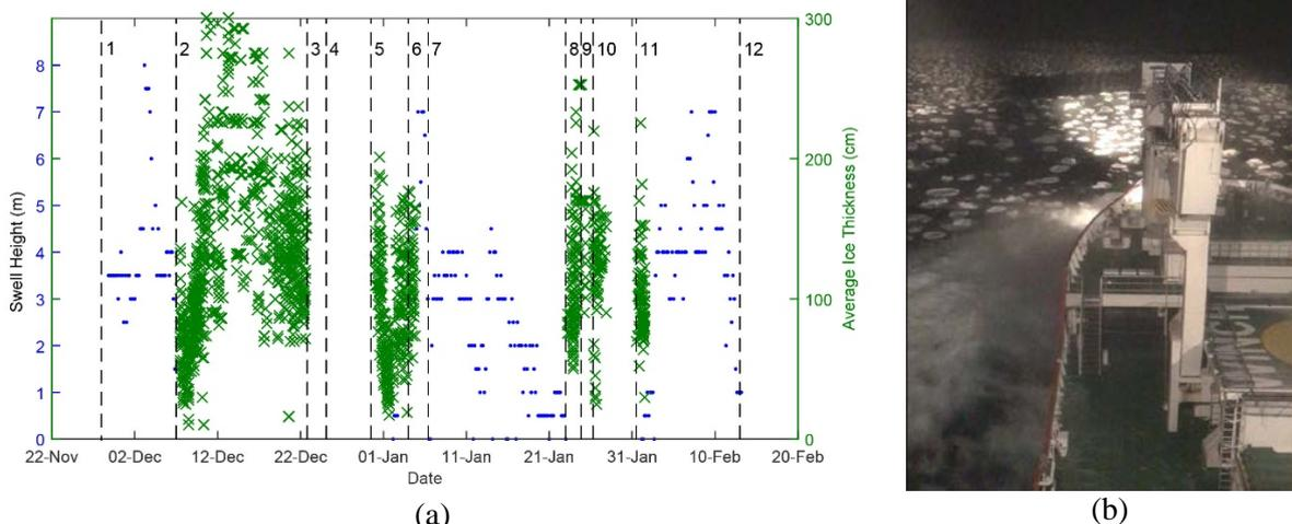
Fig.10: (a) Example of observed wave height and ice thickness on an Antarctic relief voyage. (b) Wave slamming in 7 m swells as experienced in a marginal ice zone.
