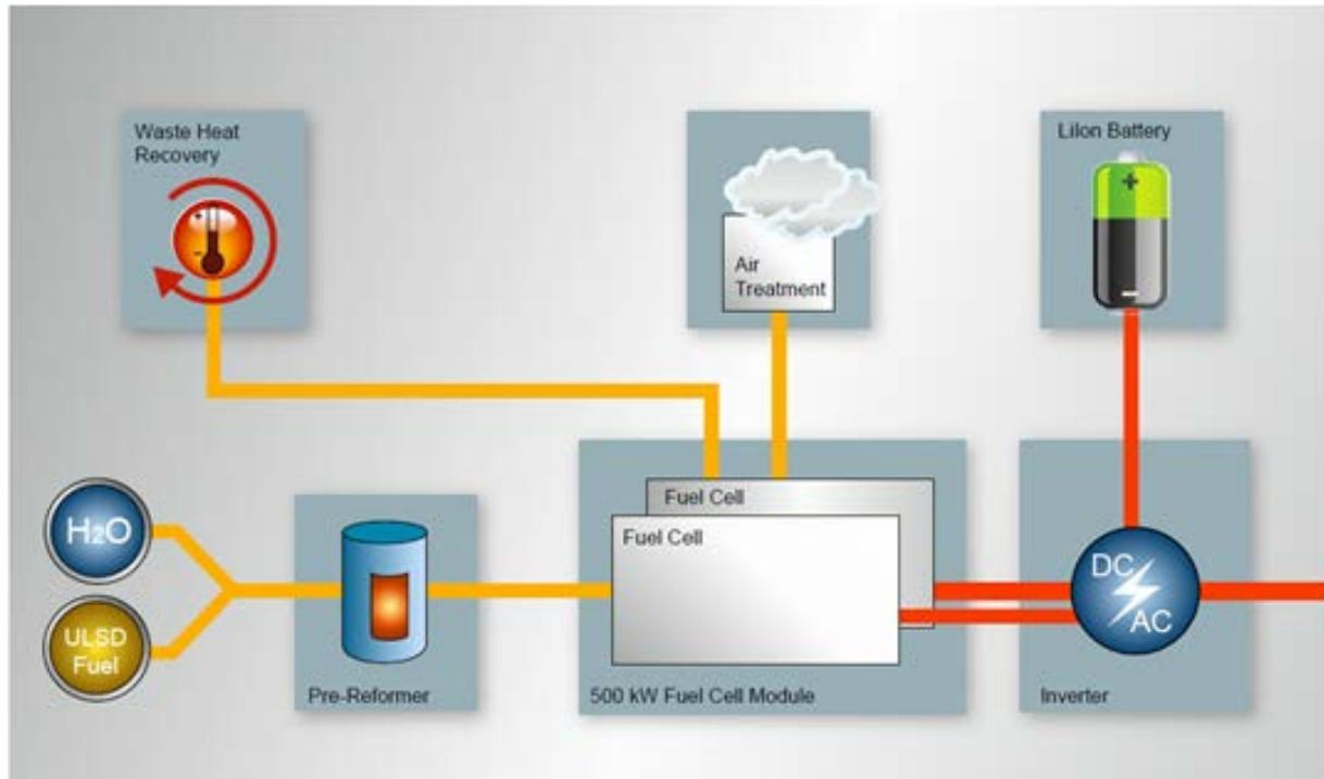
Fig.9: Simplified schematic of the proposed fuel cell system as APU
