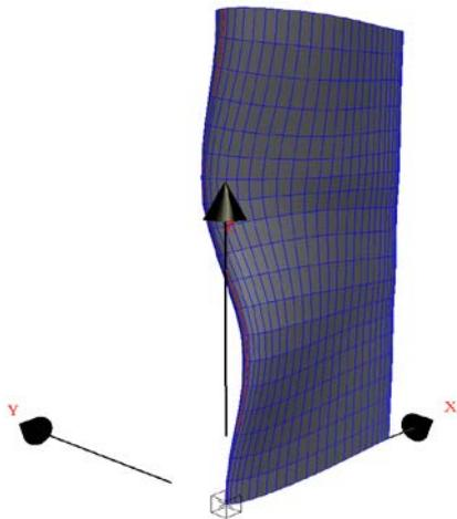
Fig.3: Exemplary twisted rudder blade
