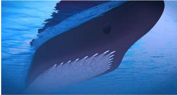
Fig.13: Air lubrication, [www.silverstream-tech.com](http://www.silverstream-tech.com)
