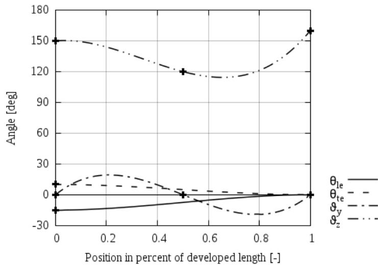
Fig.6: Faired angular parameters of the propeller blade. Points with explicitly given values are marked with a plus.
