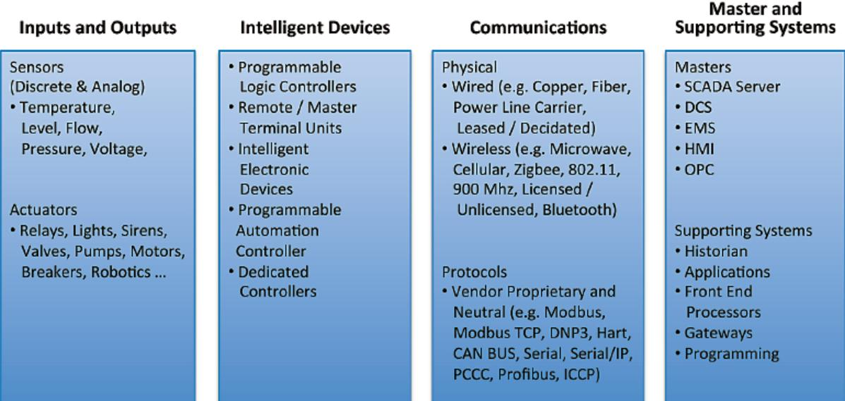
Fig.2: Typical components within an automation system, *Luallen (2011)*
