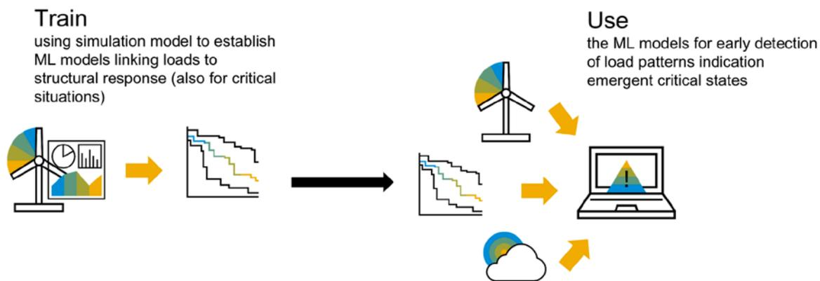
Fig.11: Using the digital twin as a simulation model for machine learning training
