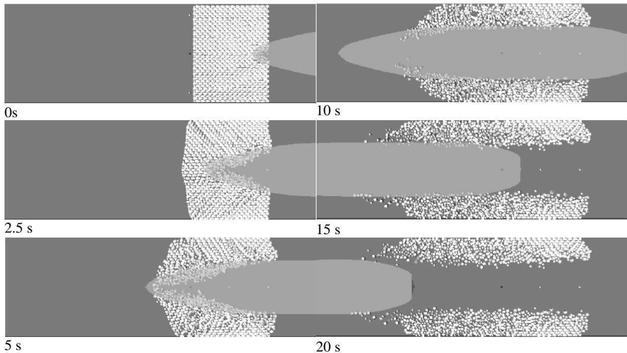
Fig. 3: Numerical simulation in brash ice with ODE, *Konno (2009)*
