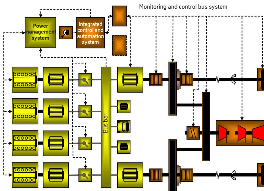
Fig.6: Mechatronic propulsion model: electric power generation and drive system (yellow) and mechanical components of propulsion train (brown)
