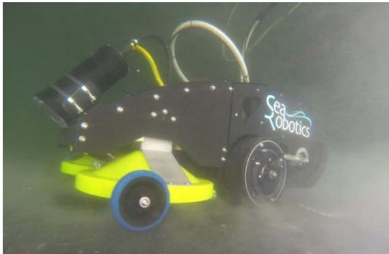
Fig.9: HullBUG cleaning robot for US Navy
