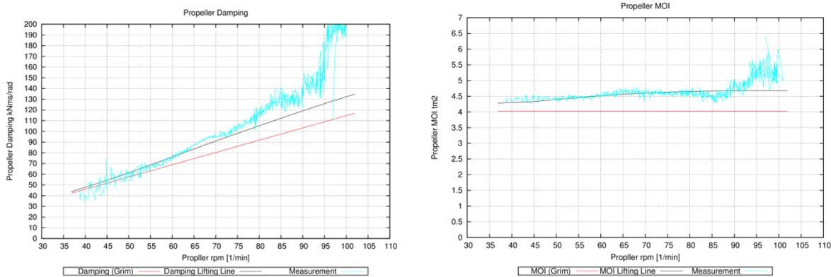
Fig.7: Measured and computed propeller MOI and damping (blue) during a sea trial run up according to *Orthmann (2016,2017)*. red: Grim's method, black: present method
