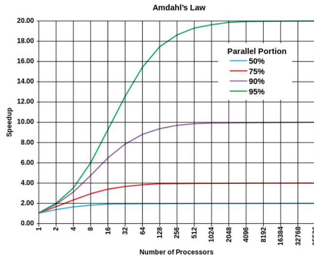
Fig.9: Amdahl's Law – Maximum speed-up as function the parallel portion of a software code
