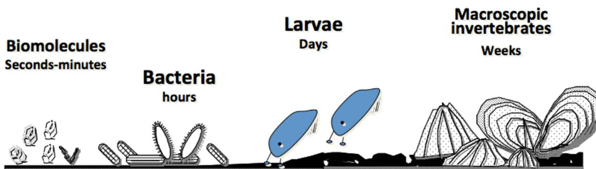
Fig.1: Progressive fouling stages, source: [changeantifouling.com](http://changeantifouling.com)
