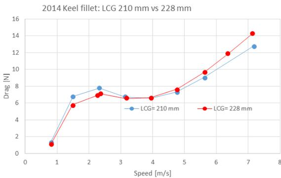
Fig.21: LCG effect for 2014 Keel fillet
