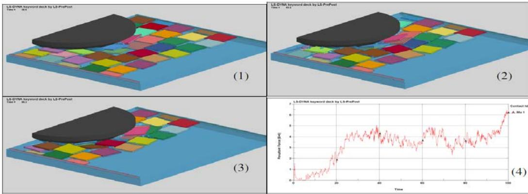
Fig. 5: Simulation of ice floes against platform using LS-DYNA, 80% ice concentration, Wang and Derradji-Aouat (2011)
