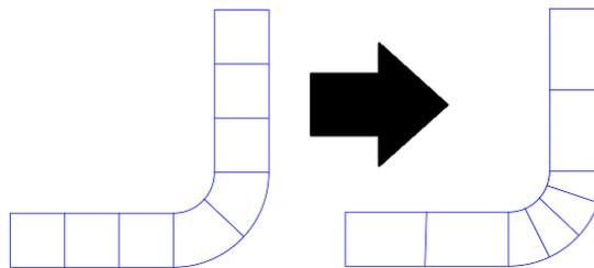
Fig.1: Example of simple r-adaptation, [http://www.cfd-online.com/Wiki/Mesh\\_adaptation](http://www.cfd-online.com/Wiki/Mesh_adaptation)
