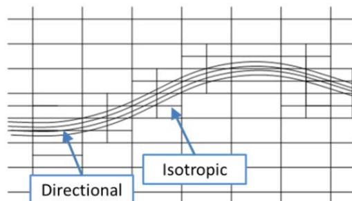
Fig.5: Directional and isotropic refinement at the free surface, *Wackers et al. (2010a)*
