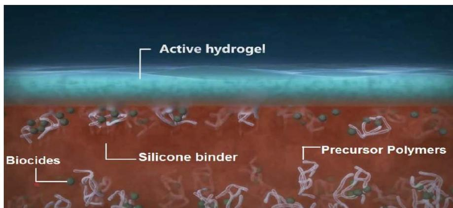
Fig.6: Working mechanism of ActiGuard®
