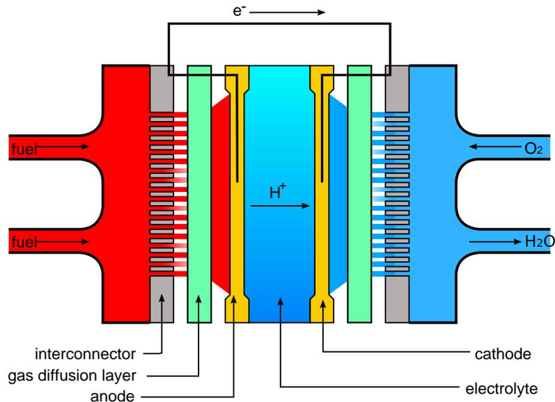
Fig.1: Principle assembly of fuel cells
