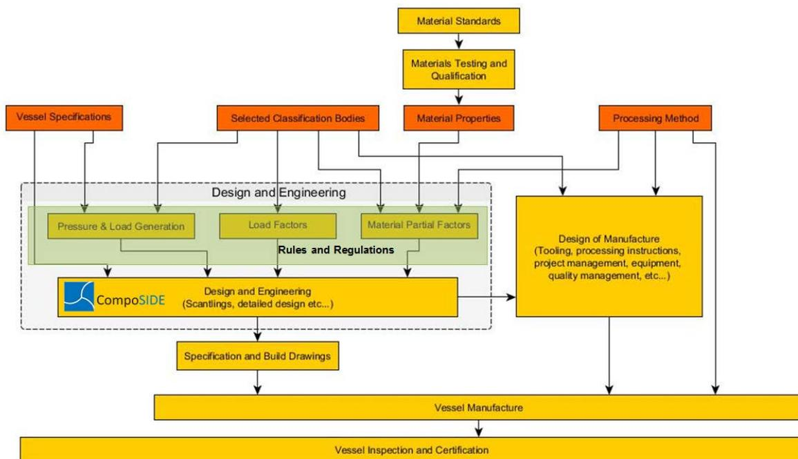
Fig.2: Composite Vessel Design Workflow
