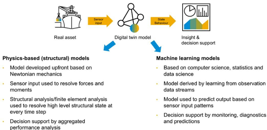
Fig.7: Physics-based vs. machine learning based digital twin solutions
