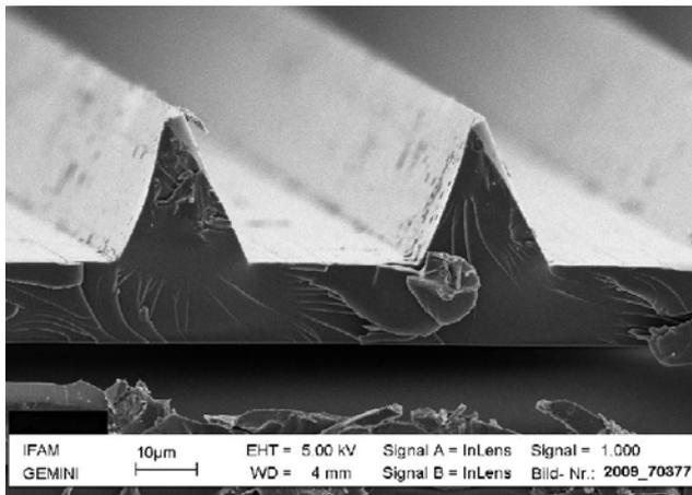
Fig.7: Riblet varnish, *Stenzel et al. (2016)*
