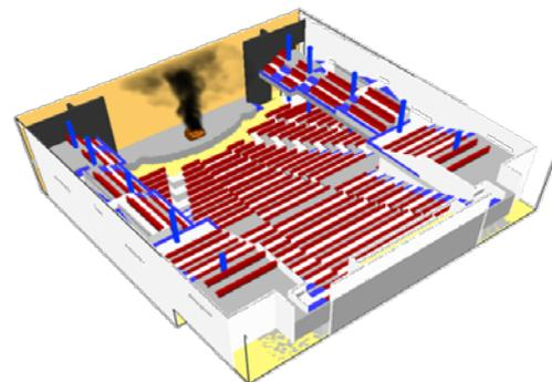
Fig.8: Fire simulation for cruise ship theater
