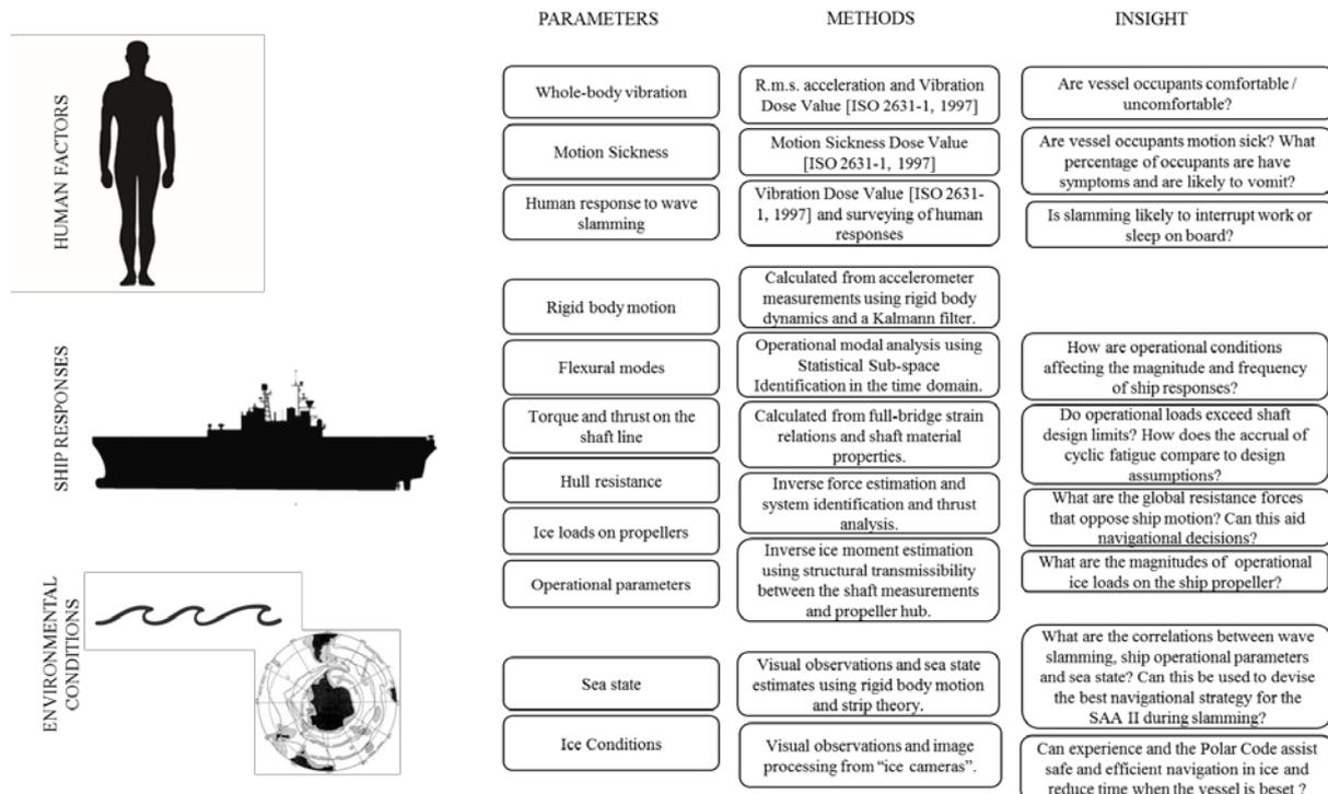
Fig.6: Real-time measurement parameters, analysis methods and anticipated insights for the SAA II
