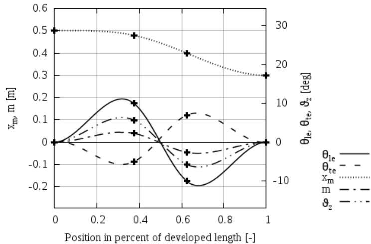
Fig.4: Faired parameters of the rudder blade. Points with explicitly given values are marked with a plus.
