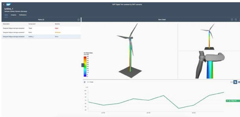
Fig.3: When selecting a wind turbine in the farm, details on structural alerts including 3D real-time visualization can be investigated.
