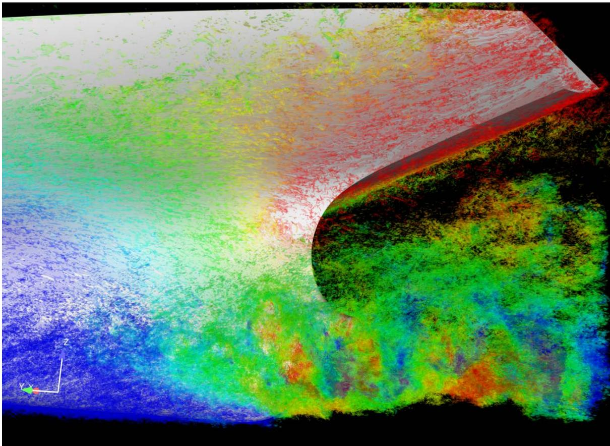
Fig.4: Large-eddy simulation of turbulence flow at ship stern, *Nishikawa (2015)*
