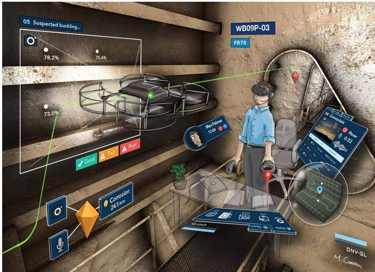
Fig. 8: Concept image of realized VR environment for remote hull surveys. (Image by Matt Corral)
