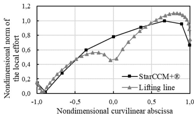
Fig.11: Nondimensional local aerodynamic force per unit length on a swept wing obtained via StarCCM+® and the lifting line method at  $5^\circ$  of incidence and  $7.5^\circ$  of sideslip.
