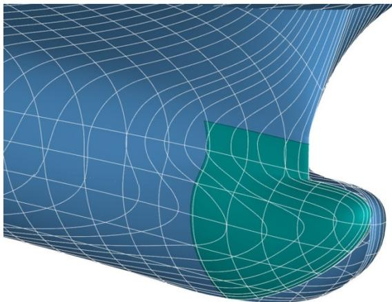
Fig.2: Original (port) and optimised bow (stb.)
