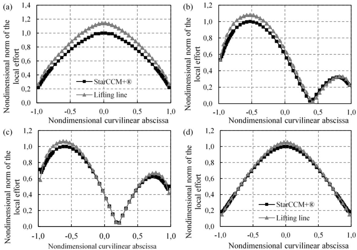
Fig. 7: Nondimensional local aerodynamic force per unit length on a kite wing obtained via StarCCM+® and the lifting line method at  $2^\circ$  of incidence and (a)  $0^\circ$  of sideslip, (b)  $7.5^\circ$  of sideslip, (c)  $15^\circ$  of sideslip, (d)  $12^\circ$  of incidence only.
