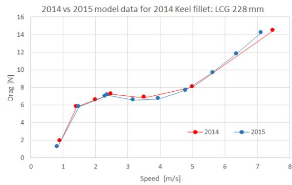
Fig.16: 2014 vs 2015 for 2014 Keel fillet drag (LCG=228 mm)
