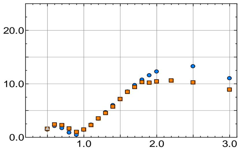
Fig.3: Amplitude of vertical acceleration at FP in regular waves
