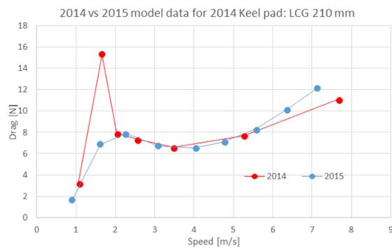
Fig.18: 2014 vs 2015 for 2014 Keel pad drag (LCG=210 mm)
