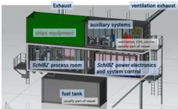
Fig.13: Standalone power supply system for technology demonstration on board
