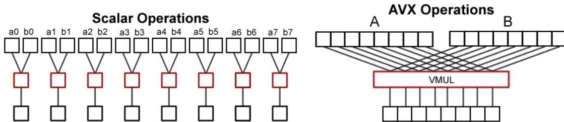
Fig.7: Eight multiplications sequentially (left), and parallel with AVX (right).
