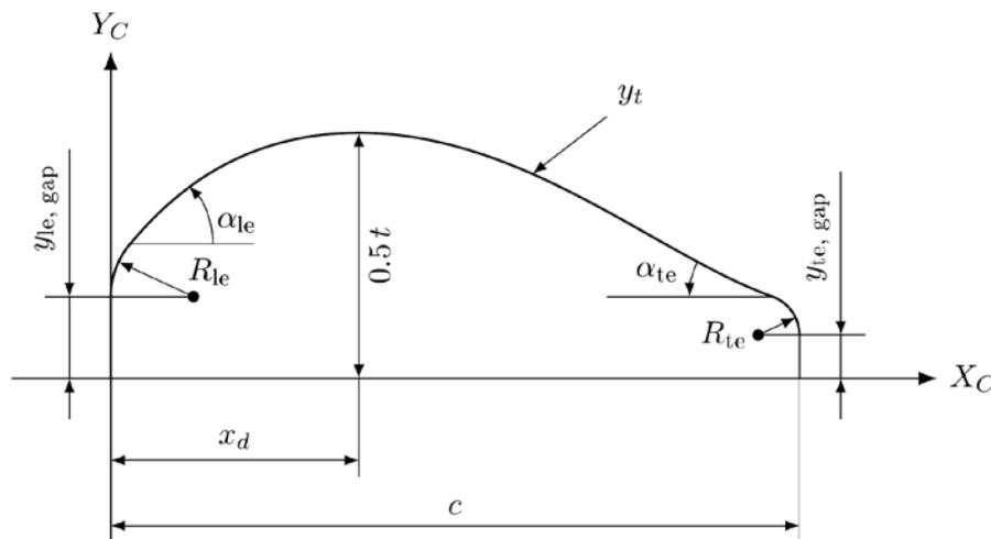
Fig.2: Parameters of the thickness line
