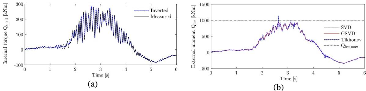
Fig.9: External propeller moment determined from measured shaft line internal torque on the SAA II through inverse methods, De Waal (2017), using Singular Value Decomposition, Generalized Singular Value Decomposition and Tikhonov regularization as proposed by *Ikonen et al. (2015)*
