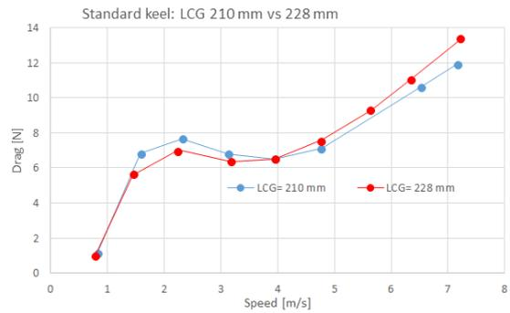
Fig.20: LCG effect for Standard keel
