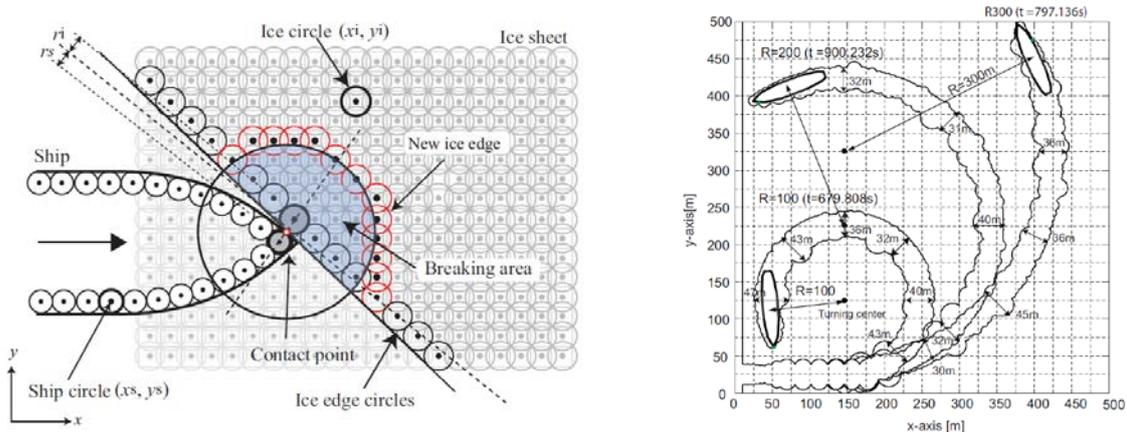
Fig. 12: Numerical ice breaking in manoeuvres, *Sawamura et al. (2010)*; circular contact detection algorithm (left) and manoeuvres (right)
