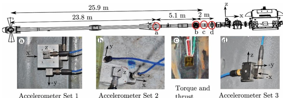
Fig.5: Accelerometers and strain gauges mounted along the shaft line for the SAA II (Adapted from technical ship drawings, source: STX Finland)
