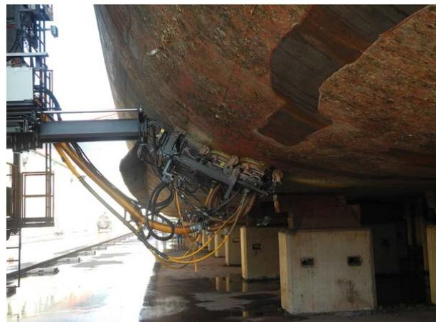
Fig.12: HTC application robot, source: Palfinger
