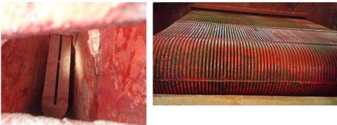
Fig.7: Boxcooler on anchor handling tug with ultrasound protection after 24 months trading West-Africa and Caribbean
