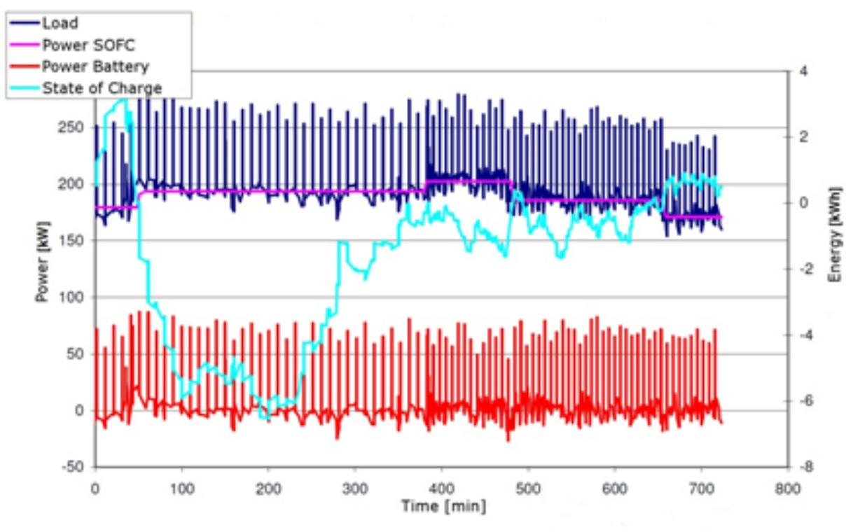
Fig.5: Detail from the load graph of the test vessel MS Forester
