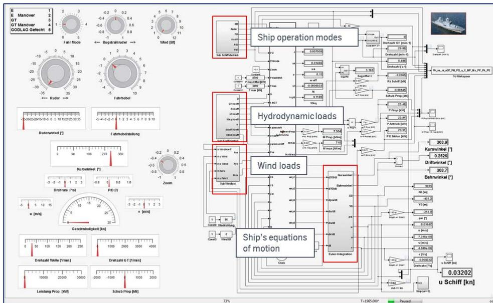
Fig.7: Matlab SIMULINK user and control interface of propulsion simulation
