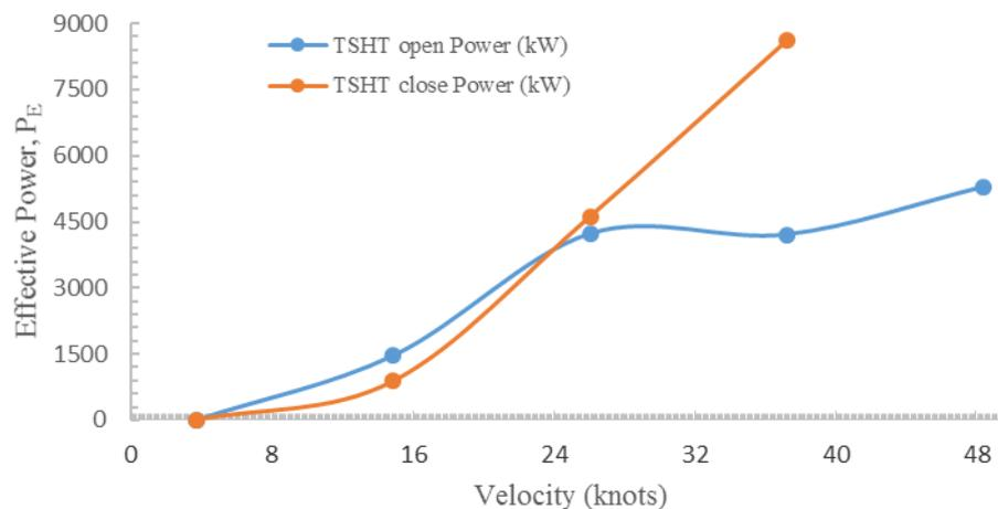
Fig.6: Effective Power (open and closed condition)
