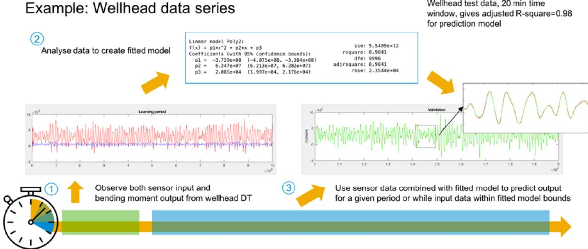
Fig.8: Computational offloading by continuous sampling and learning
