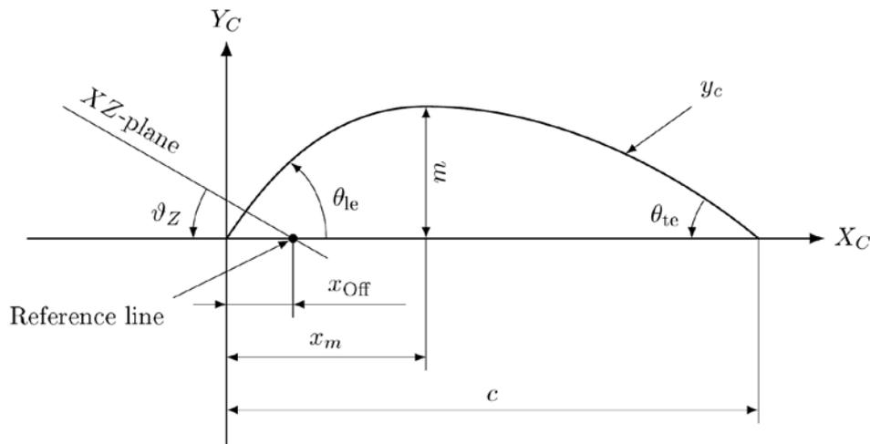
Fig.1: Parameters of the mean line
