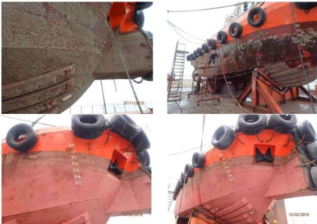
Fig.5: Tugboat without (top) and with (bottom) ultrasound protection
