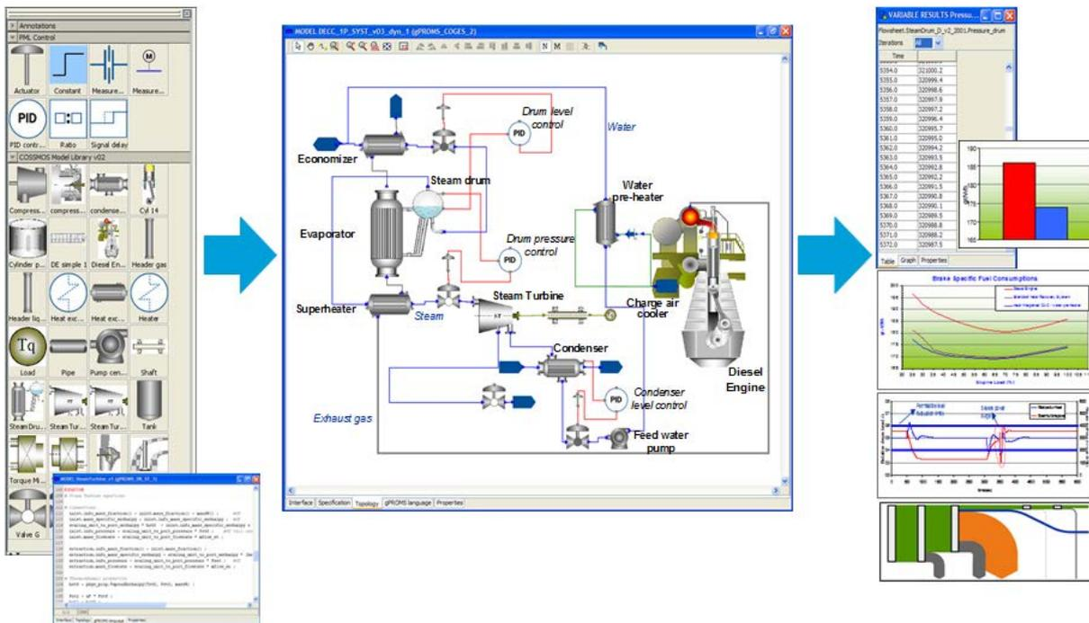
Fig.14: Energy flow simulation set up from object library to insight, Kakalis et al. (2014)
