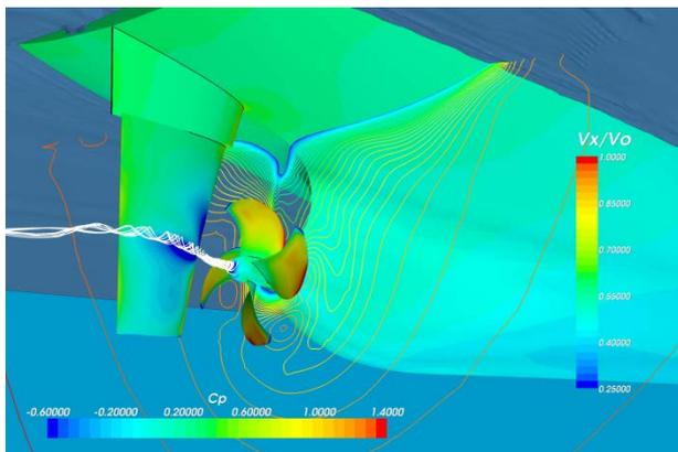
Fig.4: CFD simulation for aftbody with propeller, hull, appendage interaction
