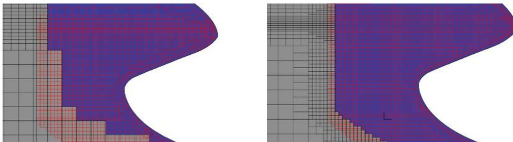
Fig.8: Initial overlapping grids (left) and adapted background mesh (right, black grid lines)
