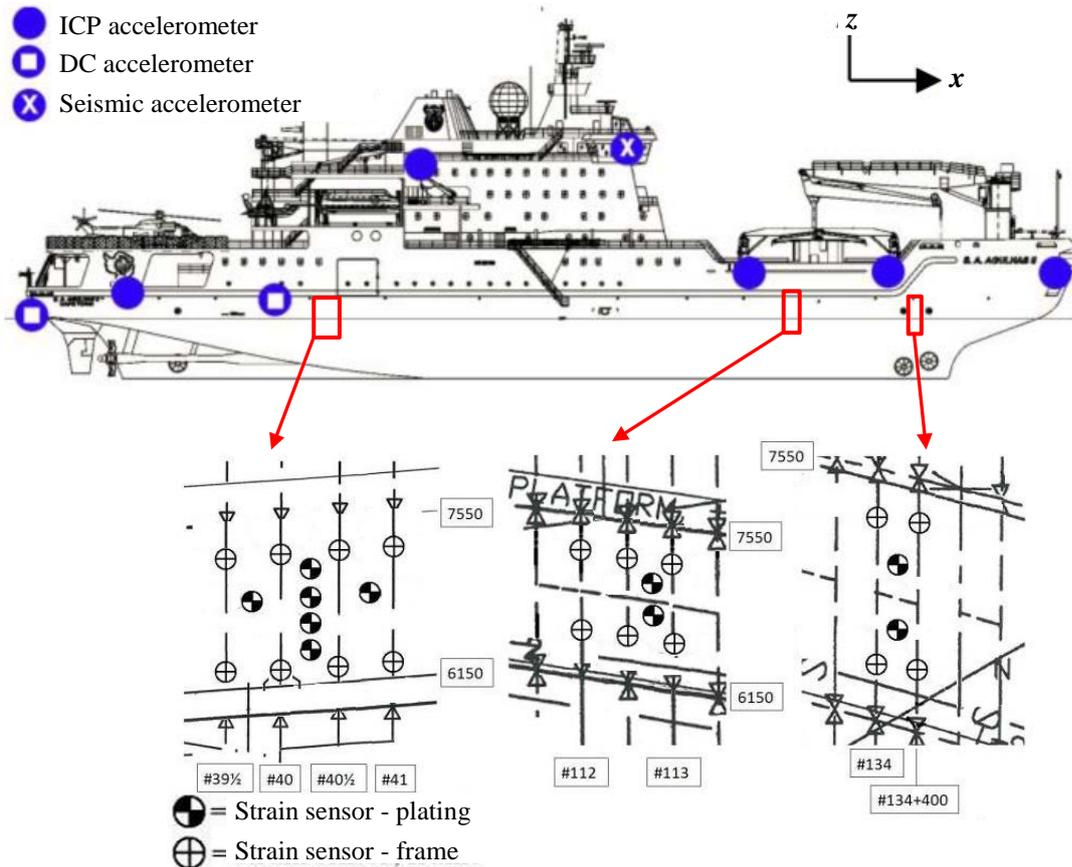
Fig.4: Network of accelerometers and strain gauge instrumentation on the ship hull at bow, bow shoulder and aft shoulder, *Kotilainen et al. (2017)*
