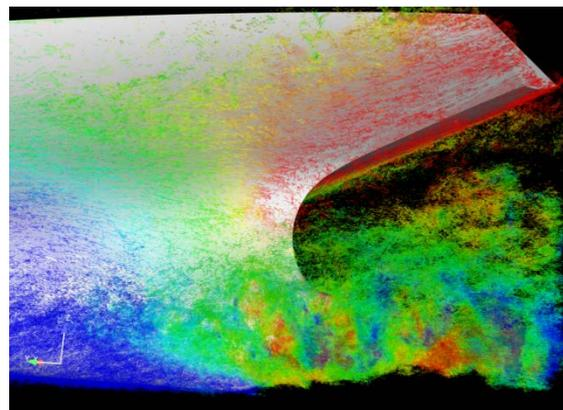
Fig.5: CFD simulation with fine resolution of turbulent structures (35 billion cells), *Nishikawa (2015)*
