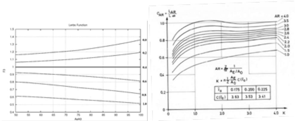
Fig.6: Recalculated correction function  $F_3$  according to LERBS (left) and correction function  $C_{AR}$  for the instationary part according to *Breslin (1970)* and *Grim (1983)* (right).
