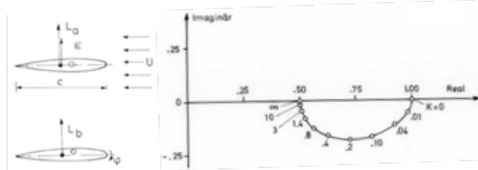
Fig.4: Definitions of flow around oscillating airfoils (left) and complex function  $C(K)$
