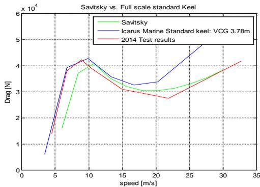
Fig.12: Savitsky drag vs. Experimental drag (LCG=3.78 m)
