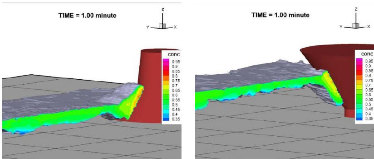
Fig.13: Numerical ice breaking simulation for upward (left) and downward (right) cone, *Barker and Sayed (2012)*
