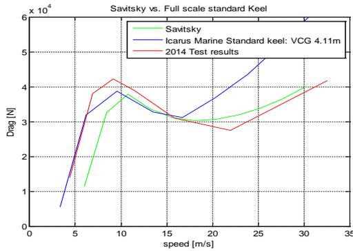
Fig.10: Savitsky drag vs. Experimental drag (LCG=4.11m)
