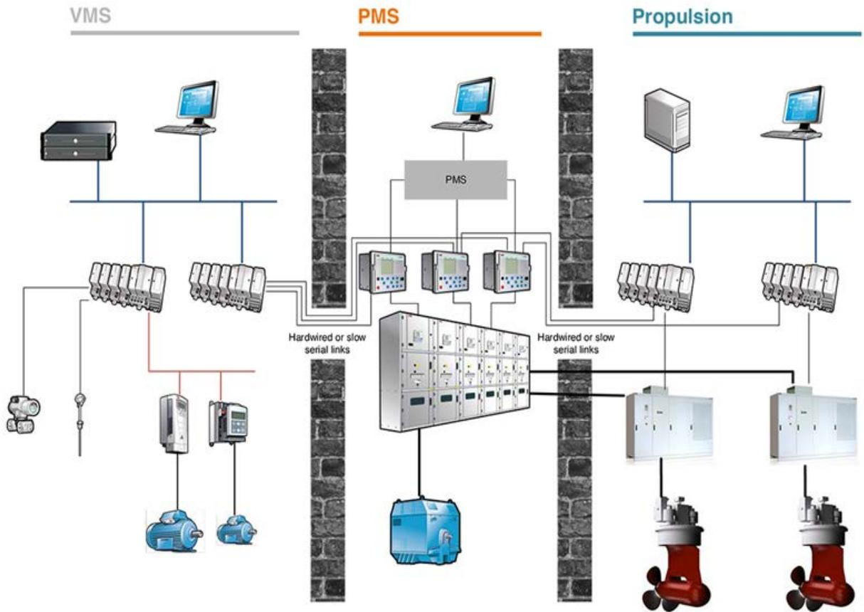
Fig.4: Traditional approach to system integration on-board, *ABB (2017)*
