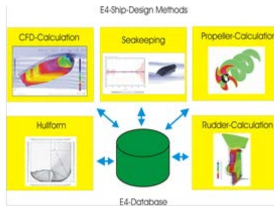
Fig.1: Principle structure of E4 ship design framework
