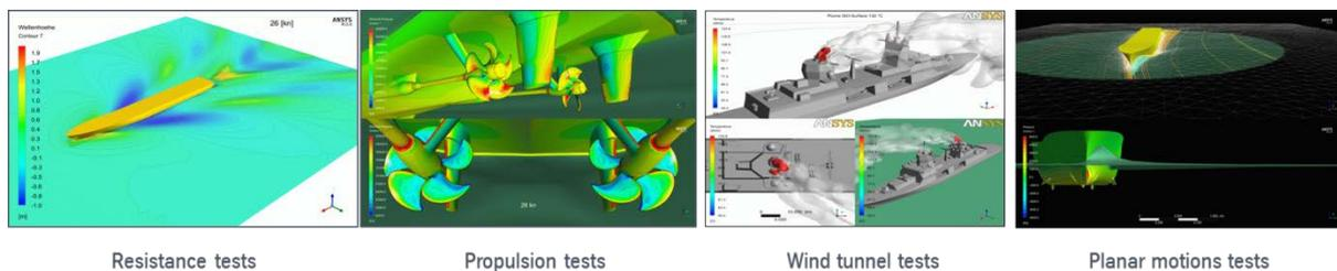
Fig.5: Preparative CFD simulations for the total system analysis
