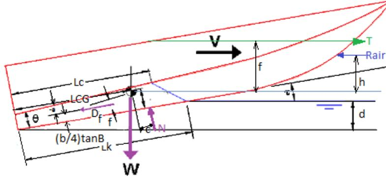
Fig.4: Icarus Marine experimental model force diagram
