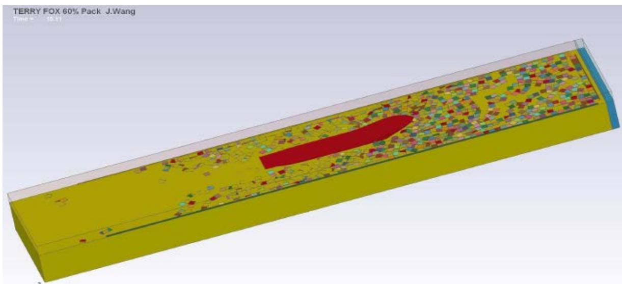
Fig. 4: Simulation of ship in brash ice using LS-DYNA, *Wang and Derradji-Aouat (2010)*
