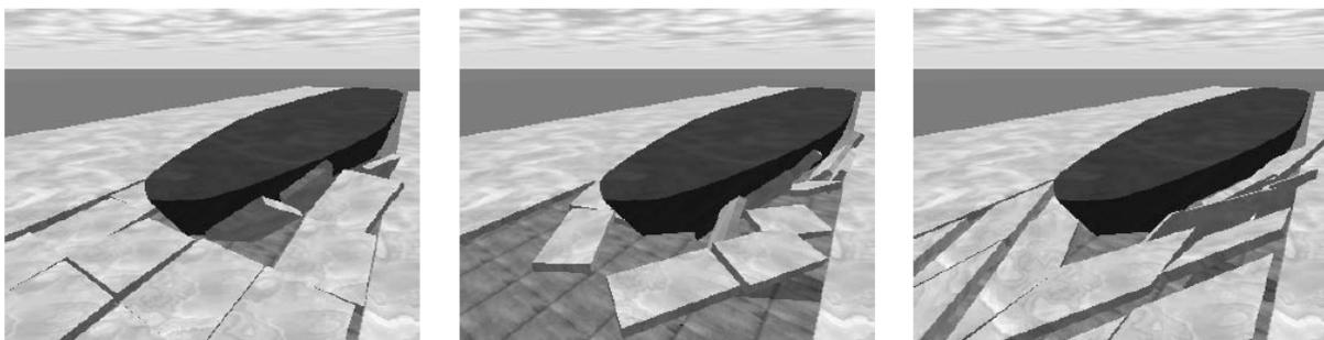
Fig. 2: Numerical simulation of pre-sawn ice test with ODE, *Konno and Mizuki (2006)*
