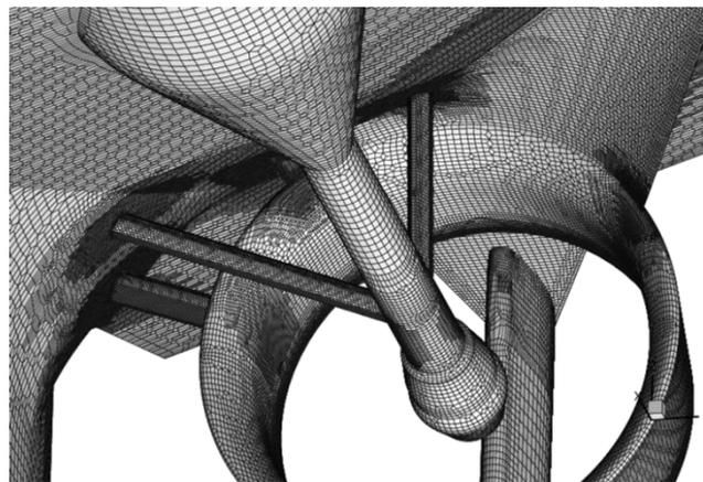
Fig.4: Example of a HEXPRESS™ mesh of ship hull with appendages
