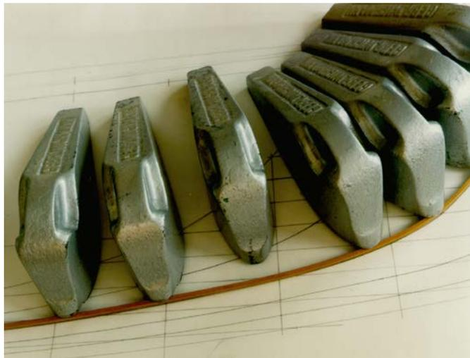
Fig.15: Cross sections and splines, ca.1700      Fig.16: Ducks and wooden spline, TU Berlin, ca. 1995
