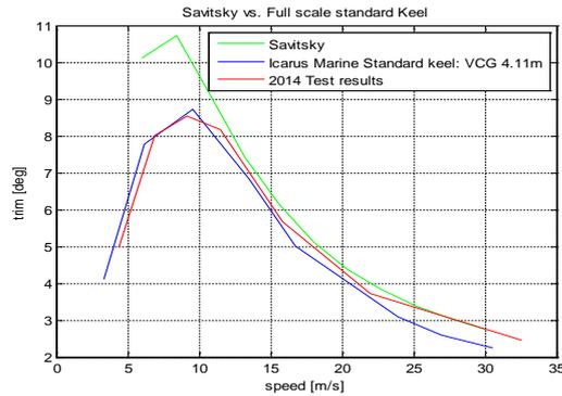
Fig.11: Savitsky trim vs. Experimental trim (LCG=4.11m)
