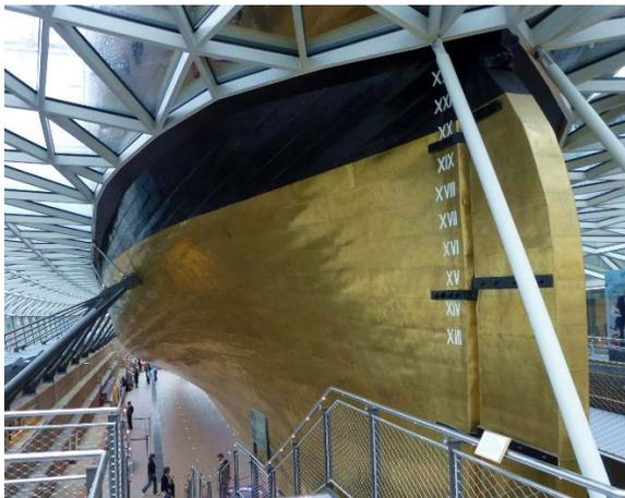
Fig.2: Copper sheathing on “Cutty Sark”, source: wikipedia
