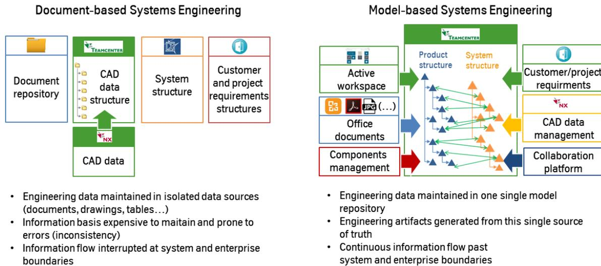
Fig.3: Document-based versus model-based systems engineering
