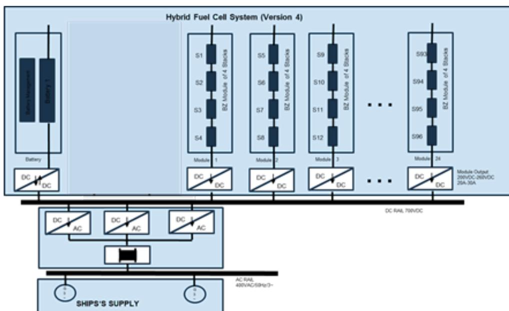
Fig.6: Basic concept of electric coupling of fuel cells and energy buffers
