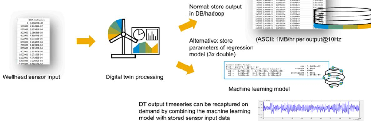
Fig.9: Limiting storage footprint by storing ML-based model parameters
