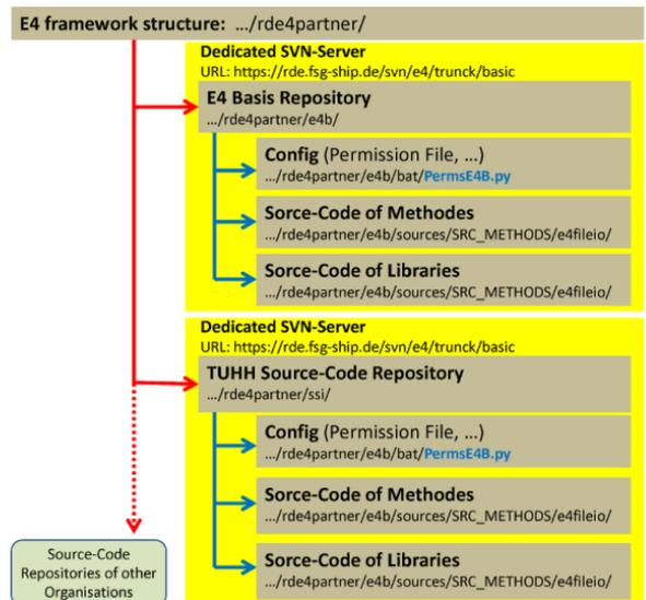
Fig.3: E4 source code structure
