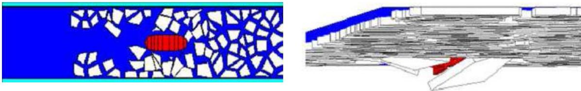
Fig. 8: Simulation in brash ice with DECICE, Lau and Simoes Ré (2006)
