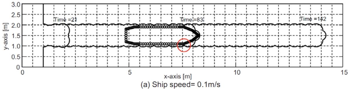
Fig. 11: Numerical ice breaking in head-on motion, *Sawamura et al. (2010)*
