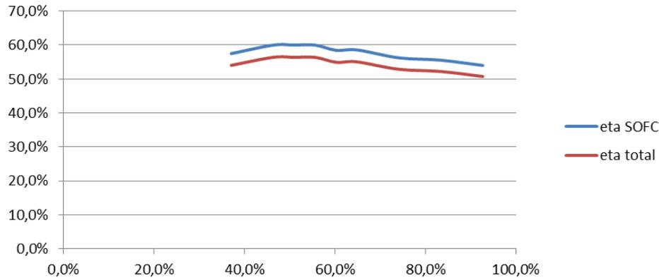
Fig.15: Efficiency curve of SchIBZ test plant (at SOFC level and including power converters)
