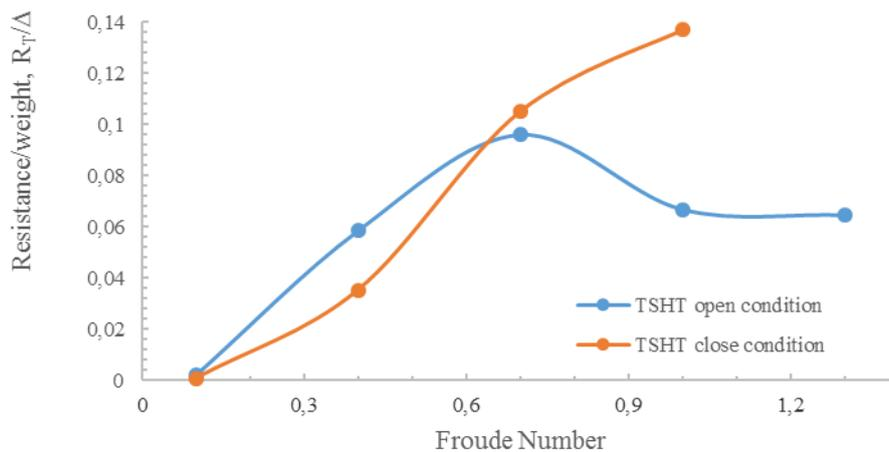
Fig.5: Resistance comparison in open and closed condition
