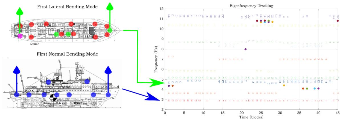
Fig.7: Migration and intermittent excitation of first lateral and vertical bending modes from full-scale measurements on the German research vessel, FS Polarstern
