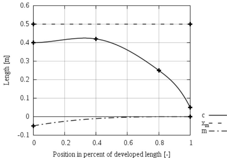
Fig.7: Faired parameters of the propeller blade with a dimension of a length. Points with explicitly given values are marked with a plus.
