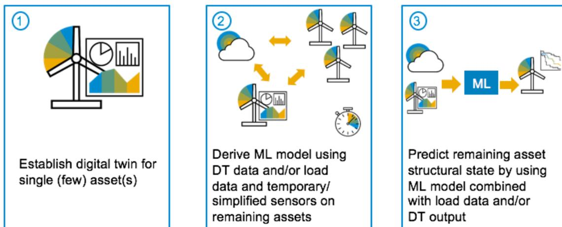
Fig.10: Combining a digital twin and machine learning for multi-asset prediction
