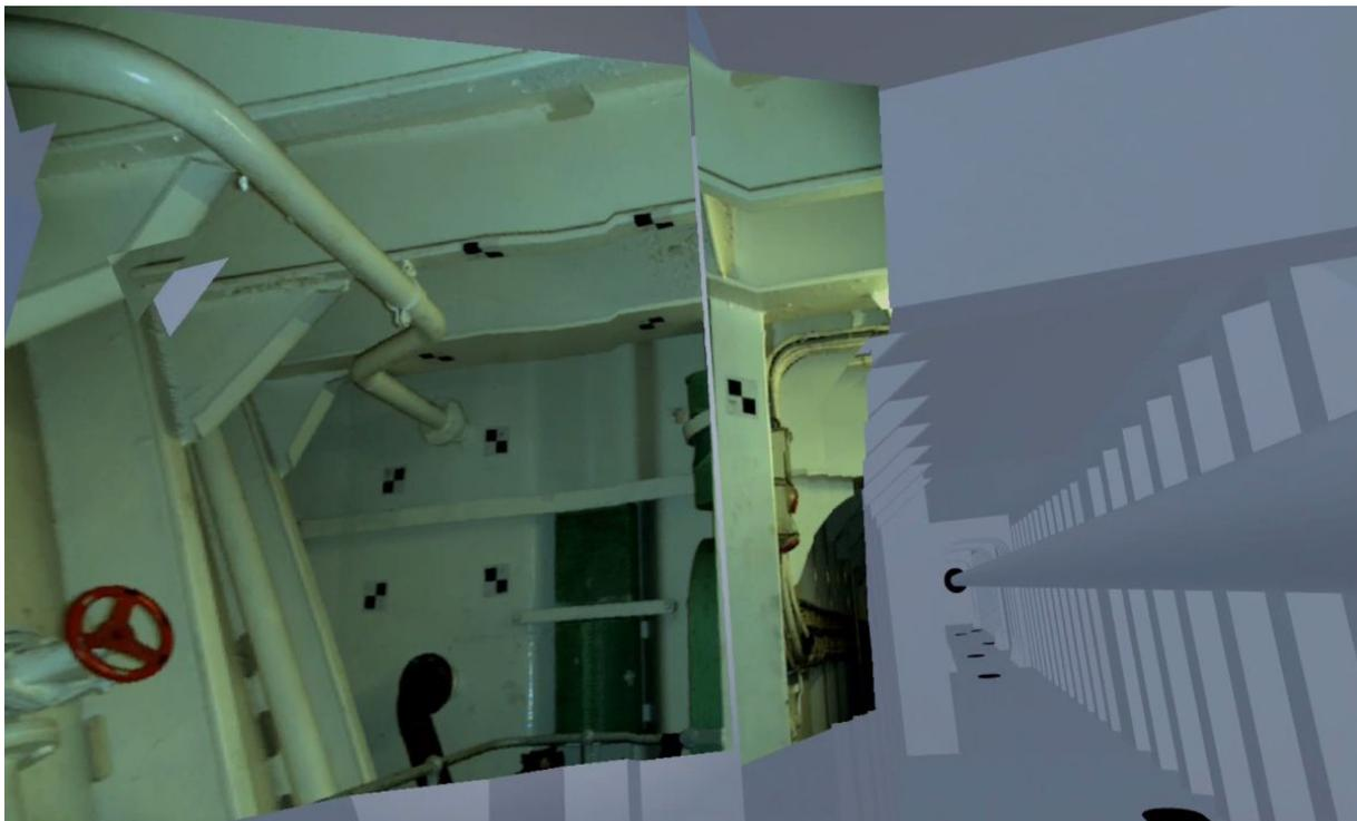
Fig.5: Inspection photo taken with IRIS inspection camera positioning the photo automatically. The photo is projected in VR onto the existing coarse 3D model.
