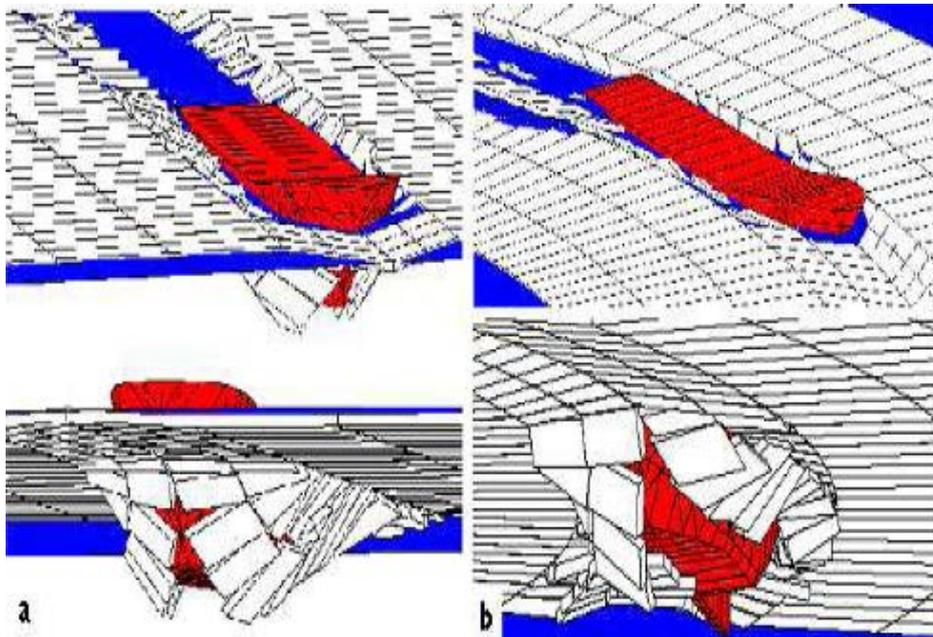
Fig. 10: Numerical ice breaking, Lau (2006)
