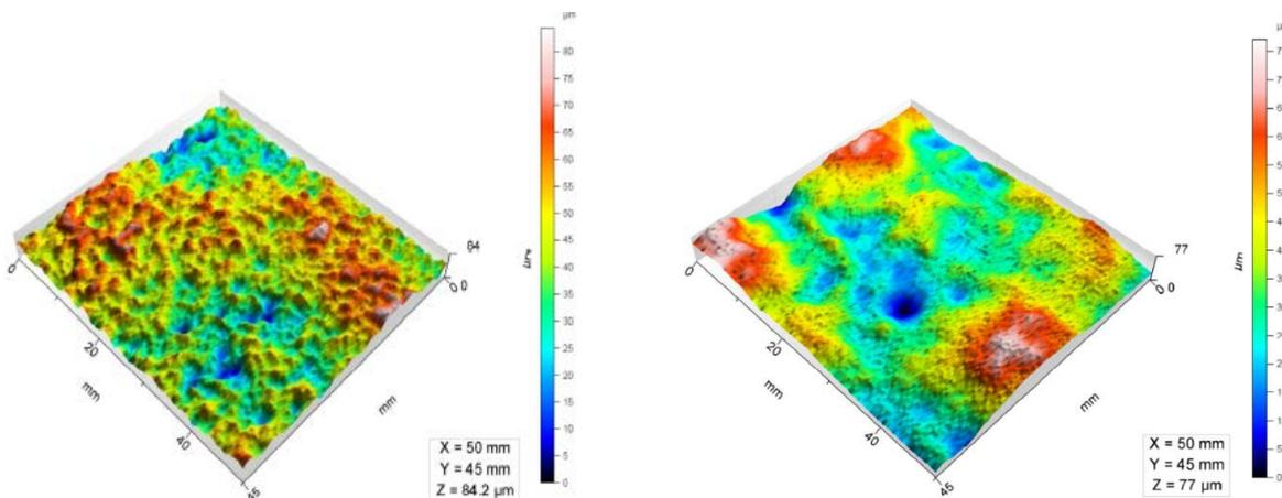
Fig.5: Roughness of SPC (Silyl acrylate) (left) and silicone-based coating (Hempaguard) (right)
