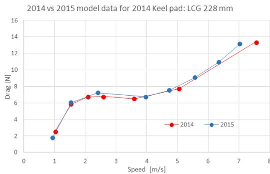
Fig.17: 2014 vs 2015 for 2014 Keel pad drag (LCG=228 mm)
