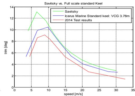
Fig.13: Savitsky trim vs. Experimental trim (LCG=3.78 m)
