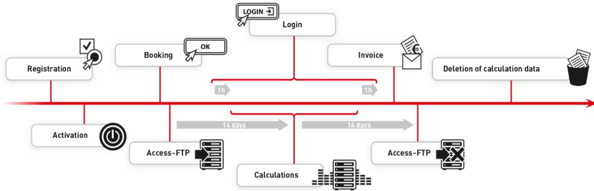
Fig.11: Time sequence of HPC allocation
