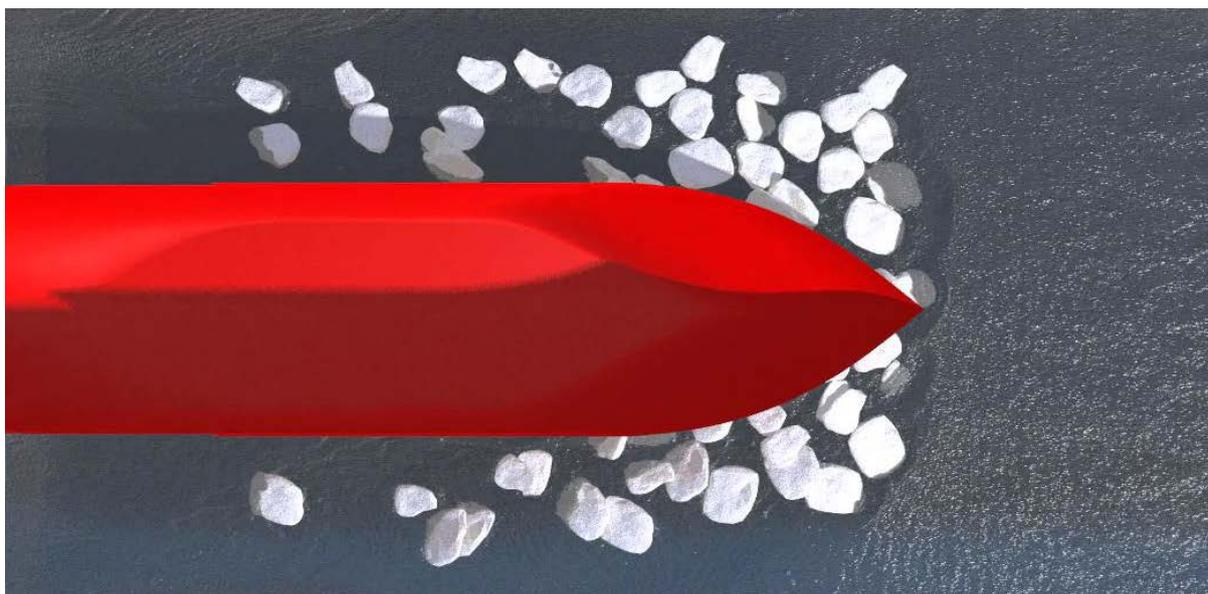
Fig. 15: Simulation of ship-ice interaction, *Mierke et al. (2015)*
