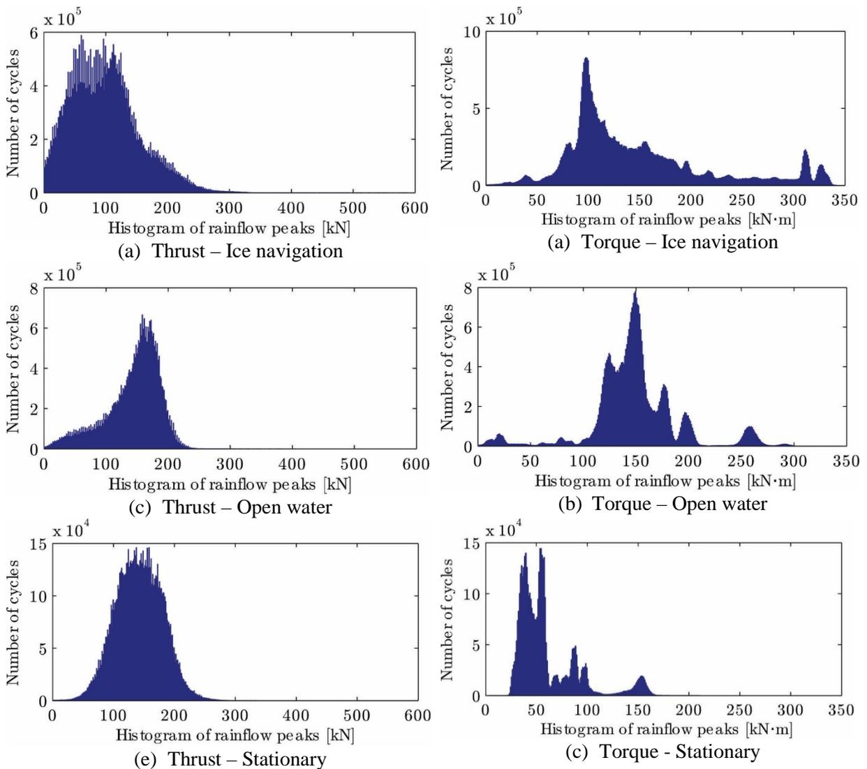
Fig.8: Thrust and torque peak rainflow cycles for the SAA II during the 2015/2016 Antarctic relief voyage, *De Waal et al. (2017)*
