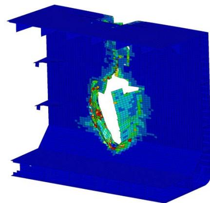
Fig.6: Collision analysis using nonlinear finite-element methods
