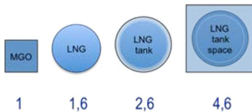
Fig.2: Bunker space needed for the same energy content with gas oil and LNG
