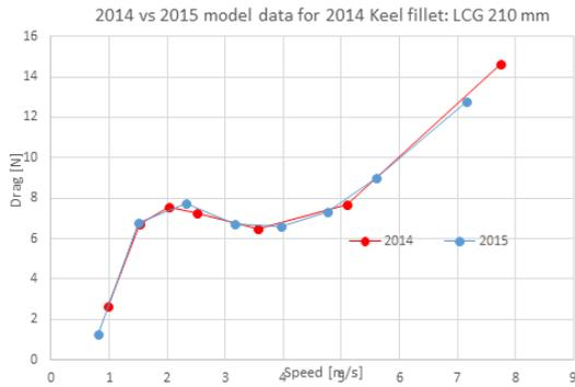
Fig.15: 2014 vs 2015 for 2014 Keel fillet drag (LCG = 210 mm)
