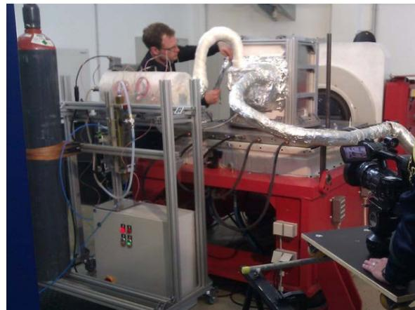
Fig.8: Vibration test at a shaker, ©sunfire
