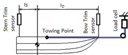
Fig.7: Model set-up
