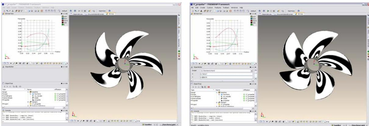
Fig.17: Variation of propeller with parametric form description, Source: CAESES
