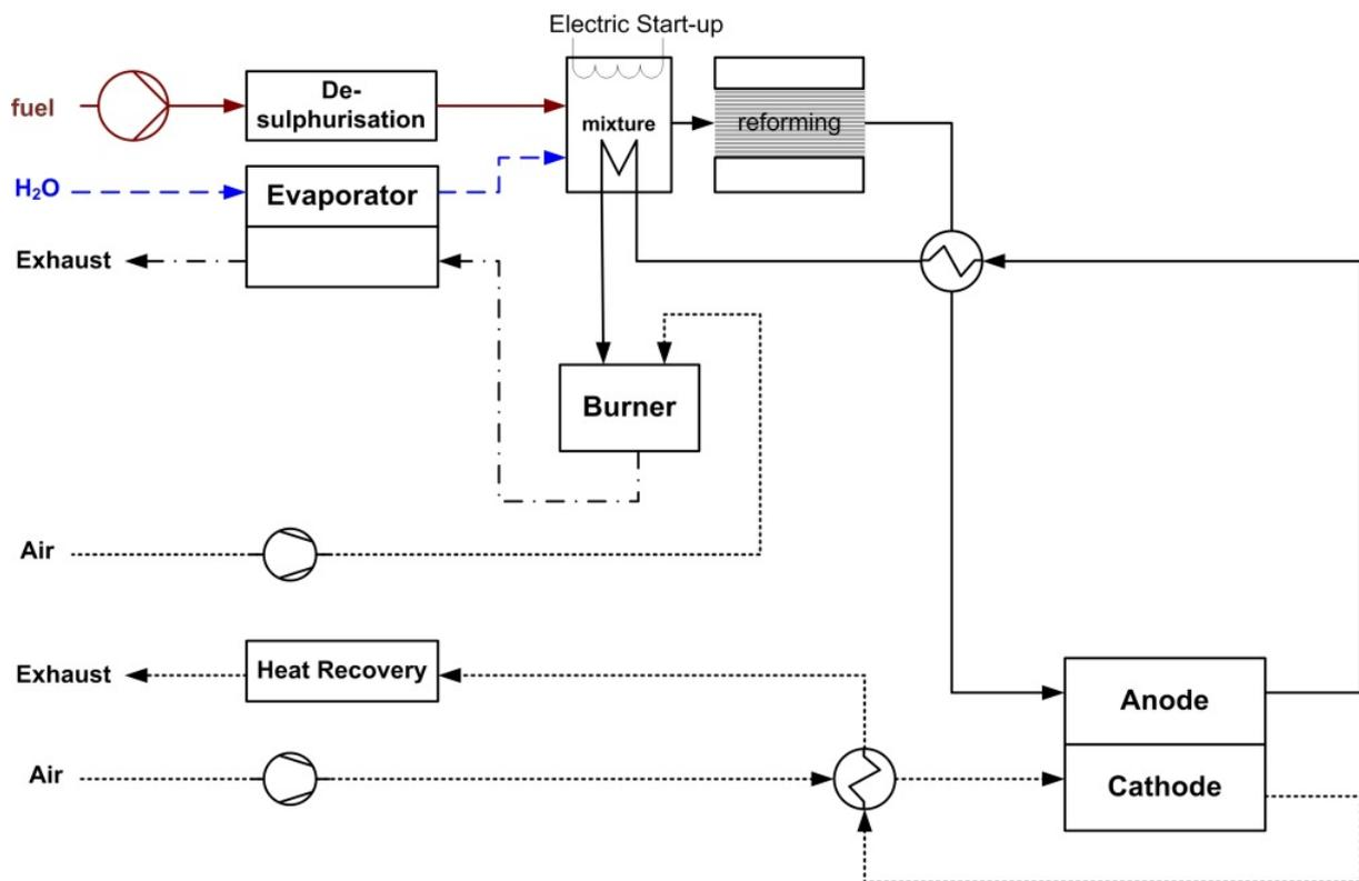
Fig.4: SOFC fuelled by road diesel, *Leites et al. (2013)*
