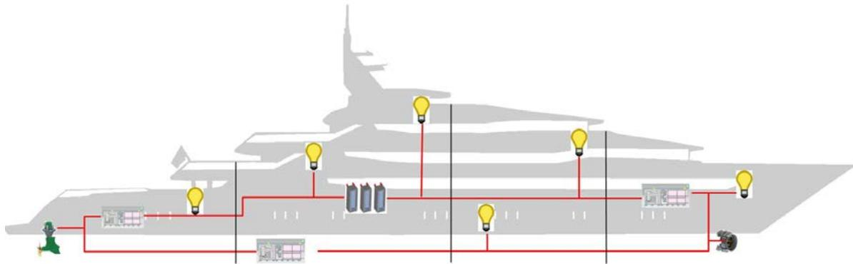
Fig.10: Concept for a distributed installation of FC systems in seagoing vessels
