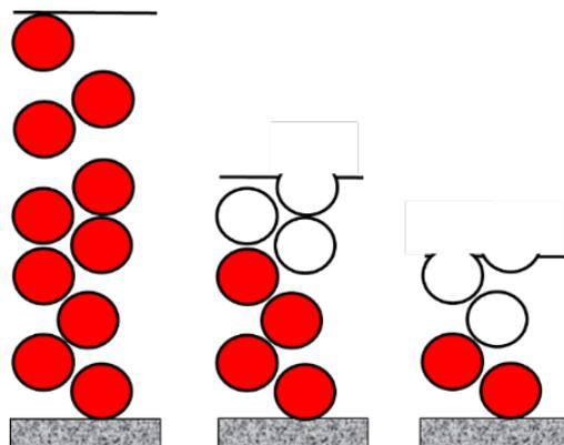
Fig.4: Principle of self-polishing co-polymers with biocides (red) and leached layer (empty circles)
