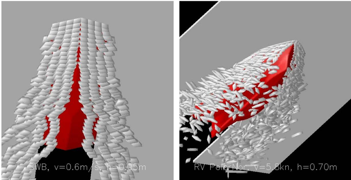
Fig. 9: Puntigliano (2003a) compares ice breaker forms capturing the differences in floe paths
