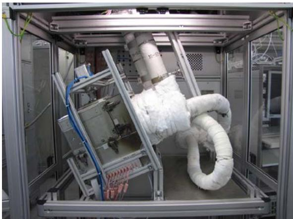
Fig.7: Test of operation at a permanent list of 22.5°, ©sunfire
