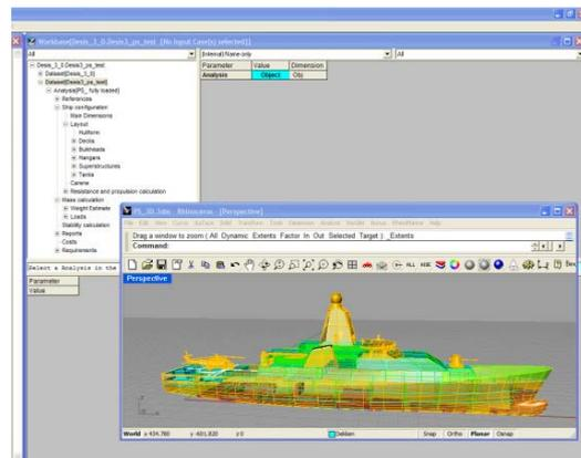
Fig.23: QUAESTOR expert system, source: MARIN
