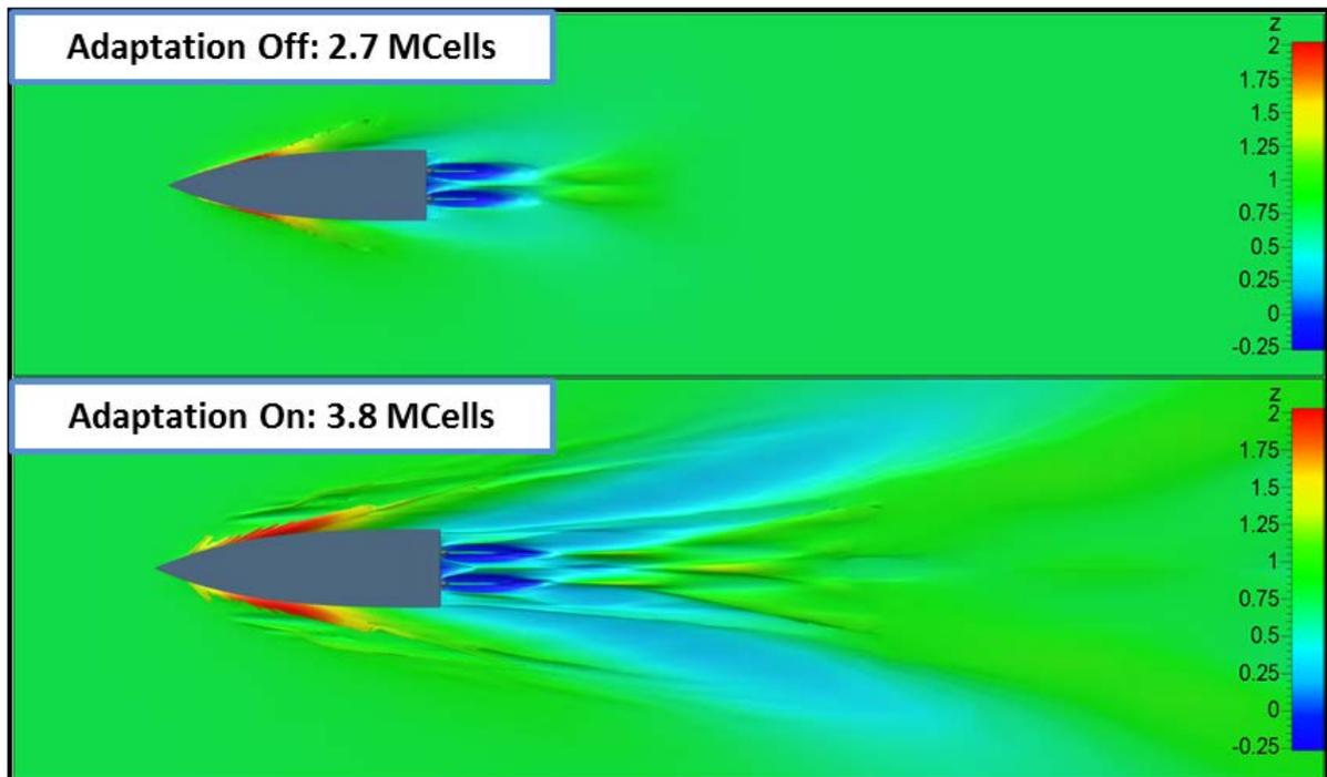
Fig.7: Wave pattern without (top) and with (bottom) mesh adaptation
