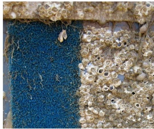
Fig.8: Flocked surface (left), source: Micanti
