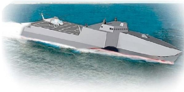
Fig.16: General Dynamics design study for US Navy littoral combat ship as trimaran
