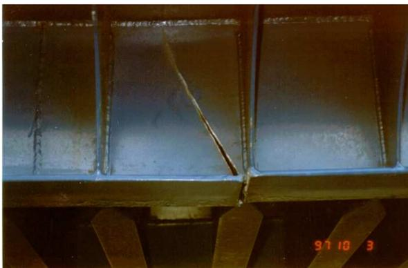
Fig. 4 Stern Ramp Damage
