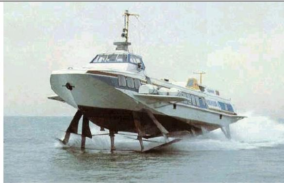
Fig.27: Typical surface-piercing hydrofoil
