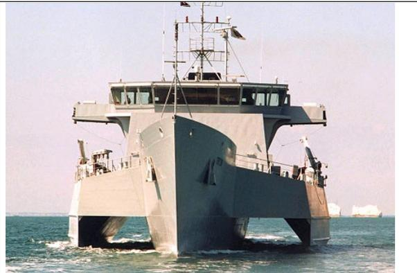
Fig.15: UK Navy Trimaran demonstrator 'Triton'
