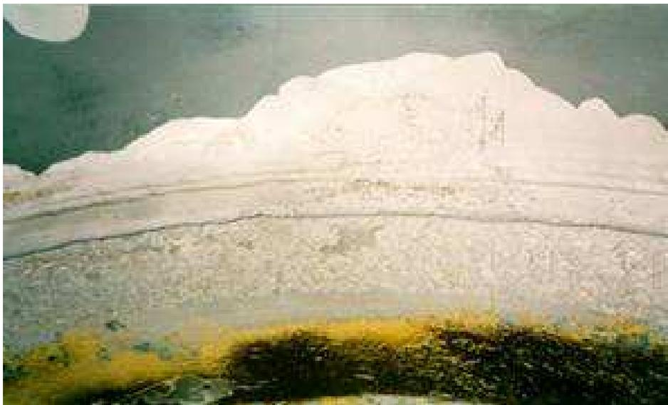
Fig. 3 Bimetallic Corrosion of Aluminum
