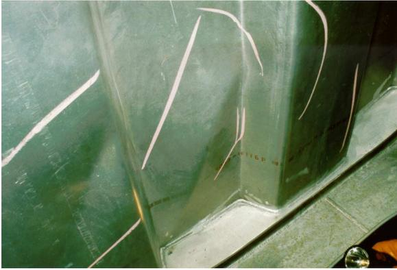
Fig. 6 Bulkhead Buckling
