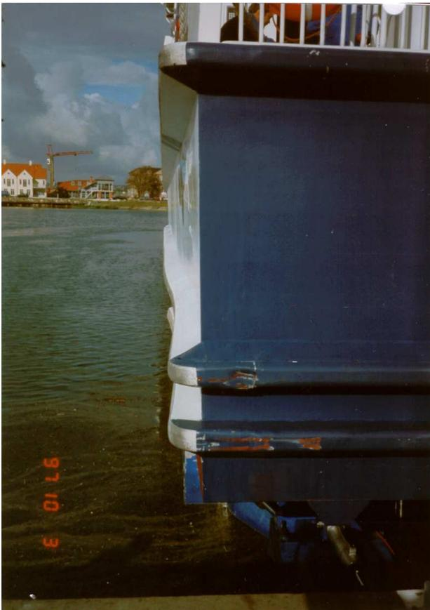
Fig. 7 Damaged Hull of HSC Catamaran
