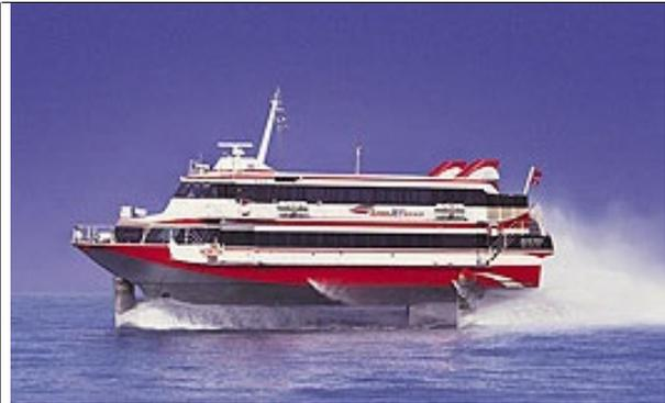
Fig.28: Jetfoil – fully submerged hydrofoils
