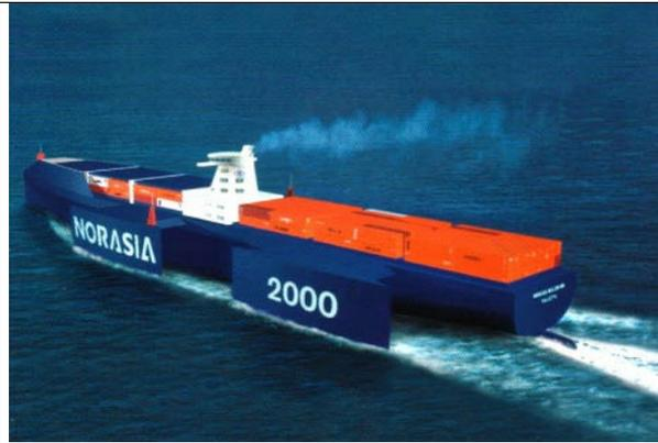
Fig.19: Pentamaran design of Nigel Gee Assoc.
