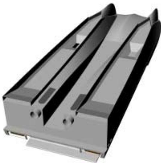
Fig.17: 24 m ASV troop transport vessel – hull form.
