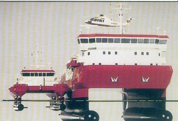
Fig.6: SWATH by Abeking+Rasmussen for pilots
