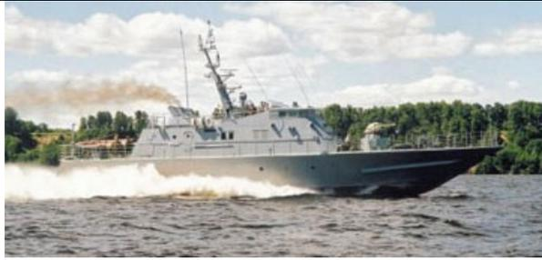
Fig.45: Sokzhoy, 55 knot Air Cavity Ship
